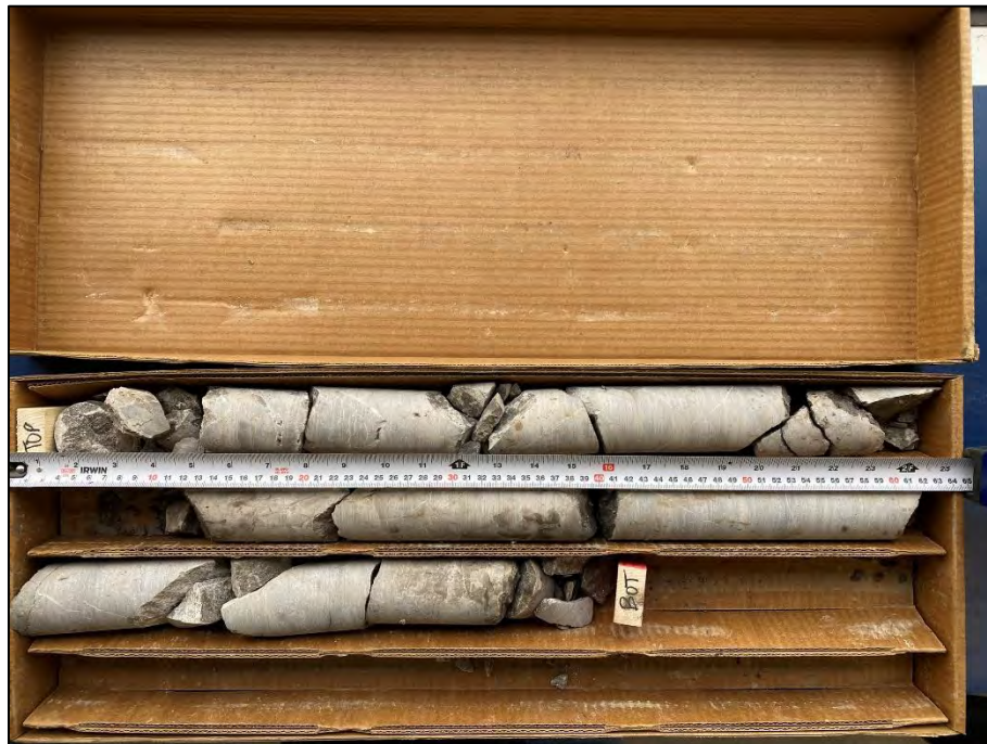
Photo 40: Photograph of RC 7 from BH 5-23 – Depth from 13.00 to 14.40 m – RQD = 75 % and REC = 100 %
