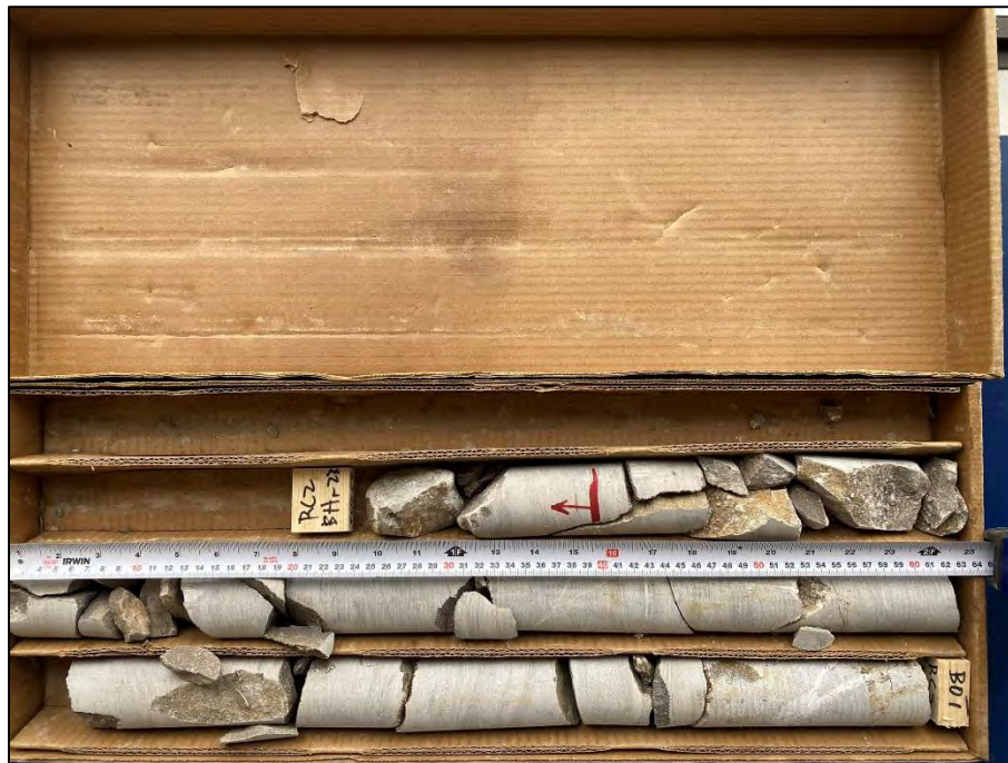
Photo 2: Photograph of RC 2 from BH 1-23 – Depth from 3.18 to 4.65 m – RQD = 72 % and REC = 100 %
