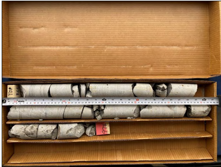
Photo 40: Photograph of RC 7 from BH 5-23 – Depth from 13.00 to 14.40 m – RQD = 75 % and REC = 100 %
