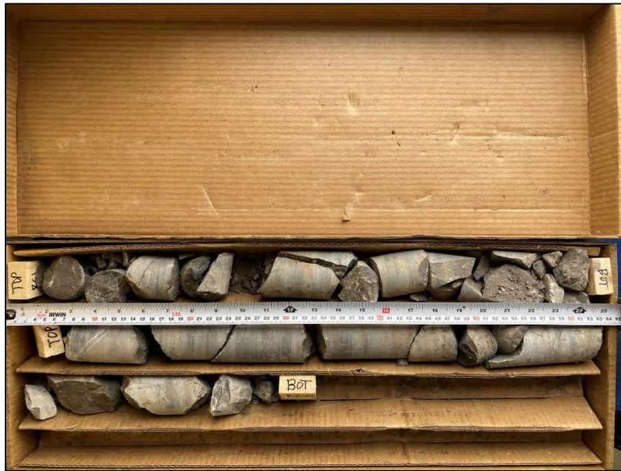
Photo 36: Photograph of RC 3 from BH 5-23 – Depth from 7.04 to 8.69 m – RQD = 49 % and REC = 100 %
