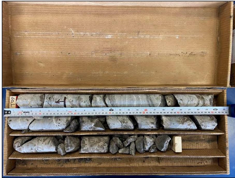
Photo 44: Photograph of RC 11 from BH 5-23 – Depth from 19.58 to 21.18 m – RQD = 52 % and REC = 100 %
