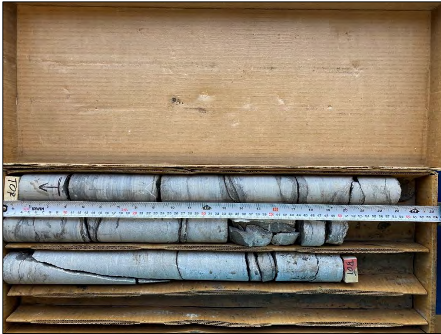
Photo 30: Photograph of RC 8 from BH 4-23 – Depth from 10.62 to 12.12 m – RQD = 86 % and REC = 100 %
