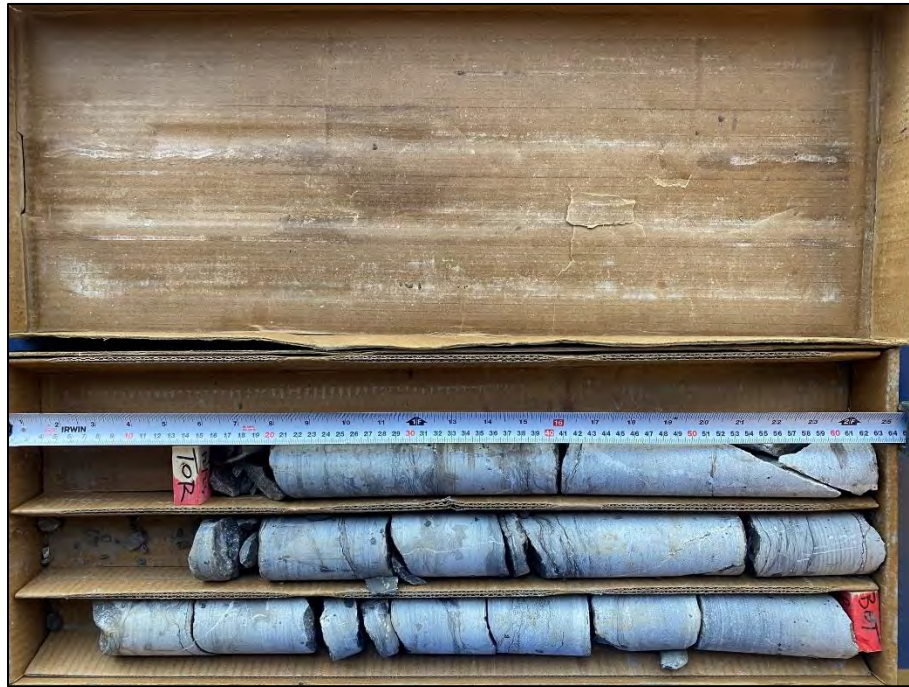
Photo 16: Photograph of RC 5 from BH 2-23 – Depth from 7.67 to 9.17 m – RQD = 59 % and REC = 100 %
