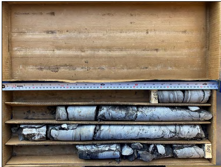
Photo 16: Photograph of RC 5 from BH 2-23 – Depth from 7.67 to 9.17 m – RQD = 59 % and REC = 100 %
