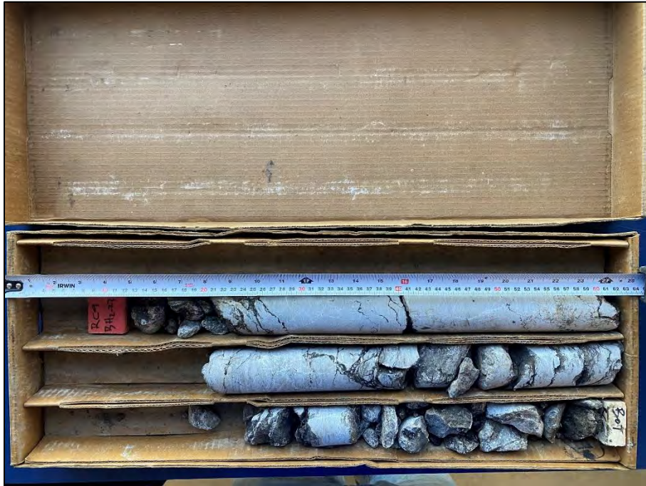
Photo 20: Photograph of RC 9 from BH 2-23 – Depth from 13.67 to 15.16 m – RQD= 47 % and REC = 85 %
