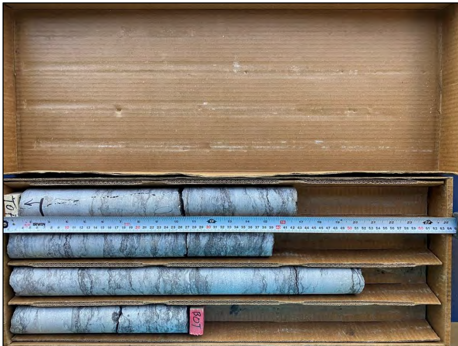
Photo 32: Photograph of RC 10 from BH 4-23 – Depth from 13.61 to 15.11 m – RQD = 100 % and REC = 100 %
