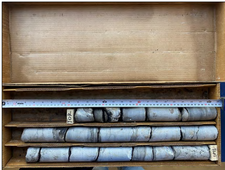
Photo 14: Photograph of RC 3 from BH 2-23 – Depth from 4.67 to 6.17 m – RQD = 73 % and REC = 100 %
