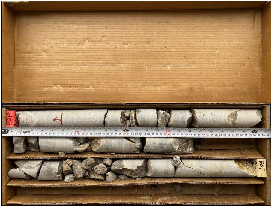
Photo 4: Photograph of RC 4 from BH 1-23 – Depth from 6.15 to 7.65 m – RQD = 59 % and REC = 100 %
