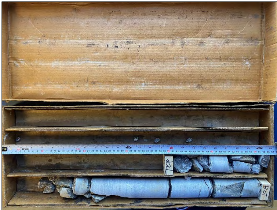
Photo 12: Photograph of RC 1 from BH 2-23 – Depth from 2.51 to 3.18 m – RQD = 62 % and REC = 100 %
