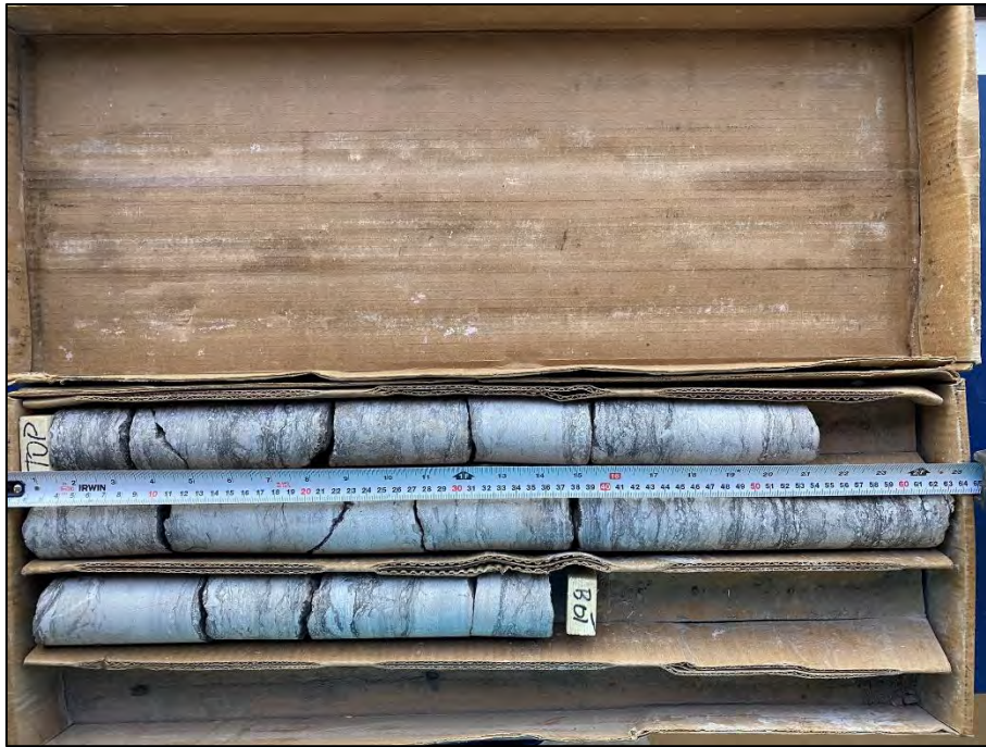
Photo 32: Photograph of RC 10 from BH 4-23 – Depth from 13.61 to 15.11 m – RQD = 100 % and REC = 100 %
