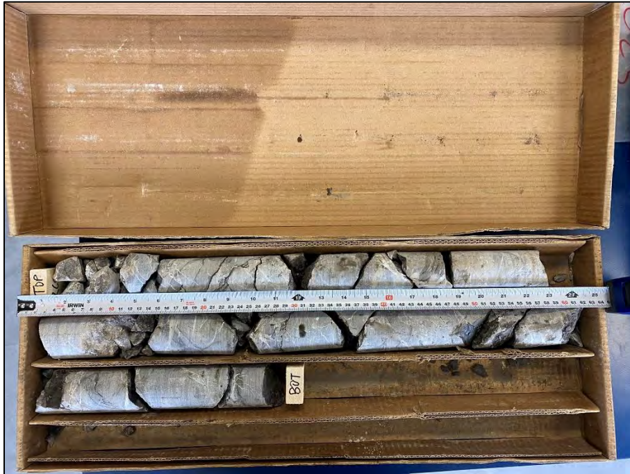
Photo 42: Photograph of RC 9 from BH 5-23 – Depth from 16.59 to 18.11 m – RQD = 57 % and REC = 100 %
