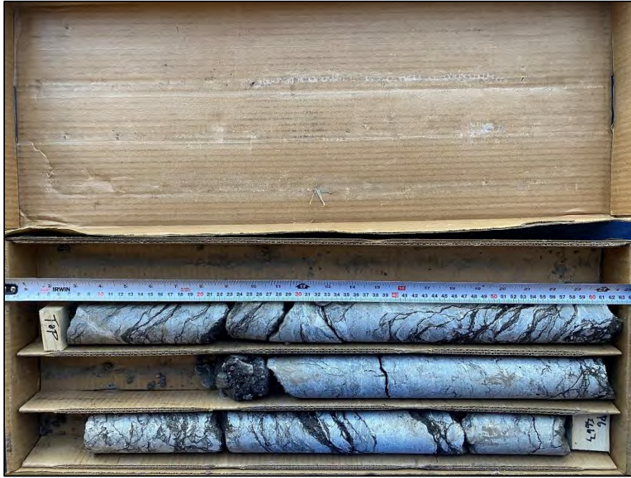
Photo 20: Photograph of RC 9 from BH 2-23 – Depth from 13.67 to 15.16 m – RQD= 47 % and REC = 85 %
