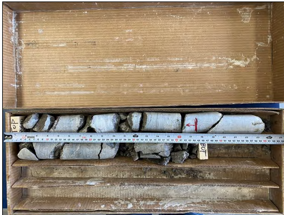
Photo 10: Photograph of RC 10 from BH 1-23 – Depth from 15.14 to 16.51 m – RQD = 59 % and REC = 100 %
