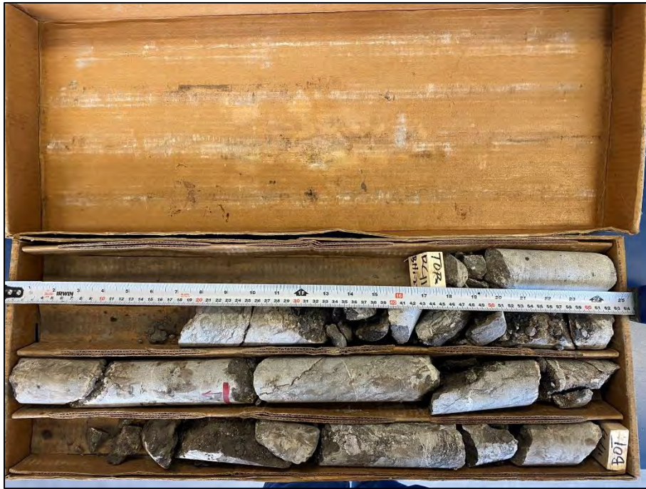
Photo 12: Photograph of RC 1 from BH 2-23 – Depth from 2.51 to 3.18 m – RQD = 62 % and REC = 100 %
