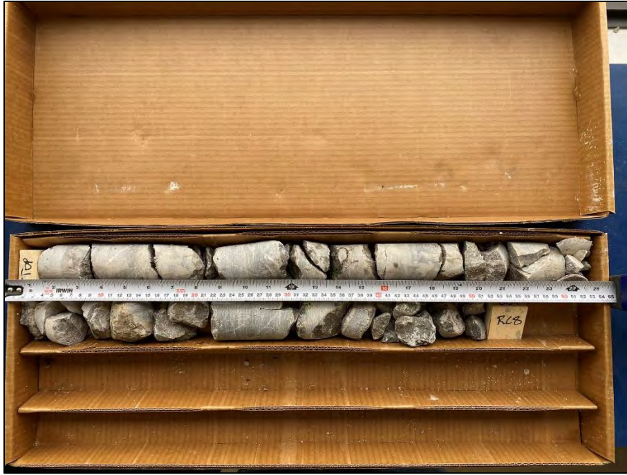
Photo 42: Photograph of RC 9 from BH 5-23 – Depth from 16.59 to 18.11 m – RQD = 57 % and REC = 100 %
