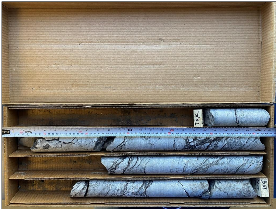
Photo 18: Photograph of RC 7 from BH 2-23 – Depth from 10.67 to 12.17 m – RQD = 93 % and REC = 100 %
