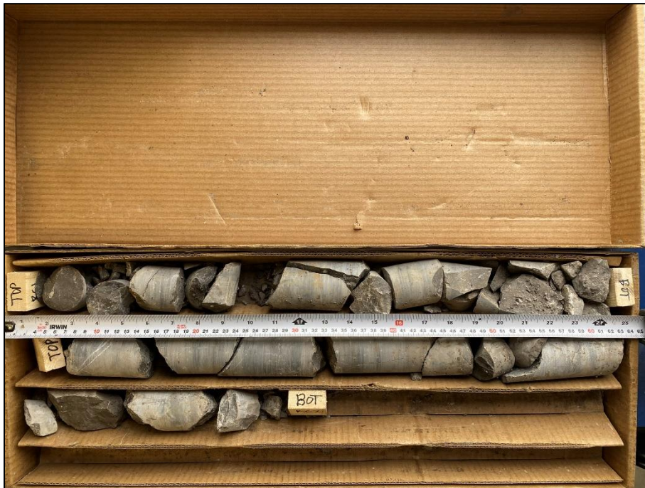
Photo 34: Photograph of RC 1 from BH 5-23 – Depth from 5.72 to 6.32 m – RQD = 0 % and REC = 100 %
