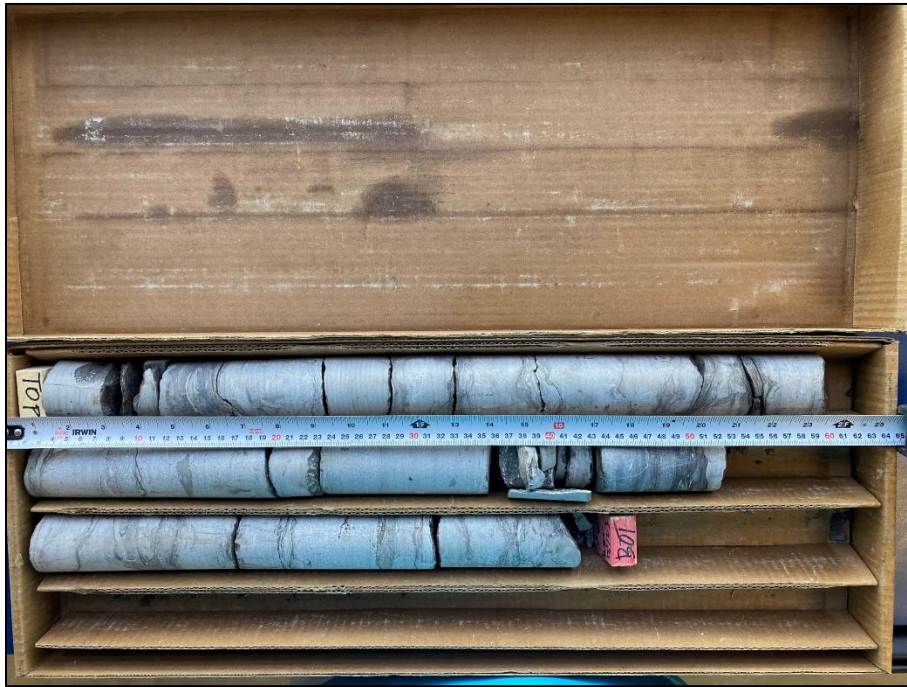
Photo 28: Photograph of RC 6 from BH 4-23 – Depth from 7.62 to 9.12 m – RQD = 97 % and REC = 100 %
