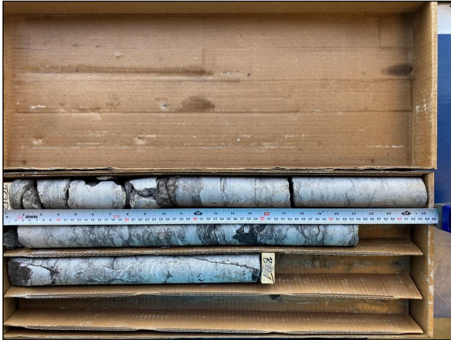
Photo 34: Photograph of RC 1 from BH 5-23 – Depth from 5.72 to 6.32 m – RQD = 0 % and REC = 100 %
