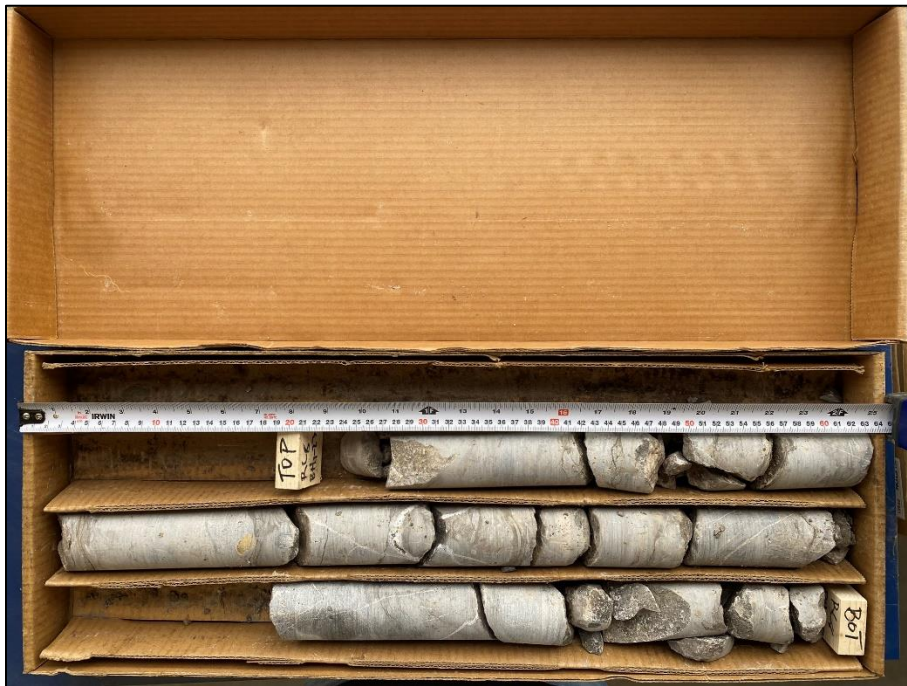
Photo 8: Photograph of RC 8 from BH 1-23 – Depth from 12.14 to 13.64 m – RQD = 56 % and REC = 93 %
