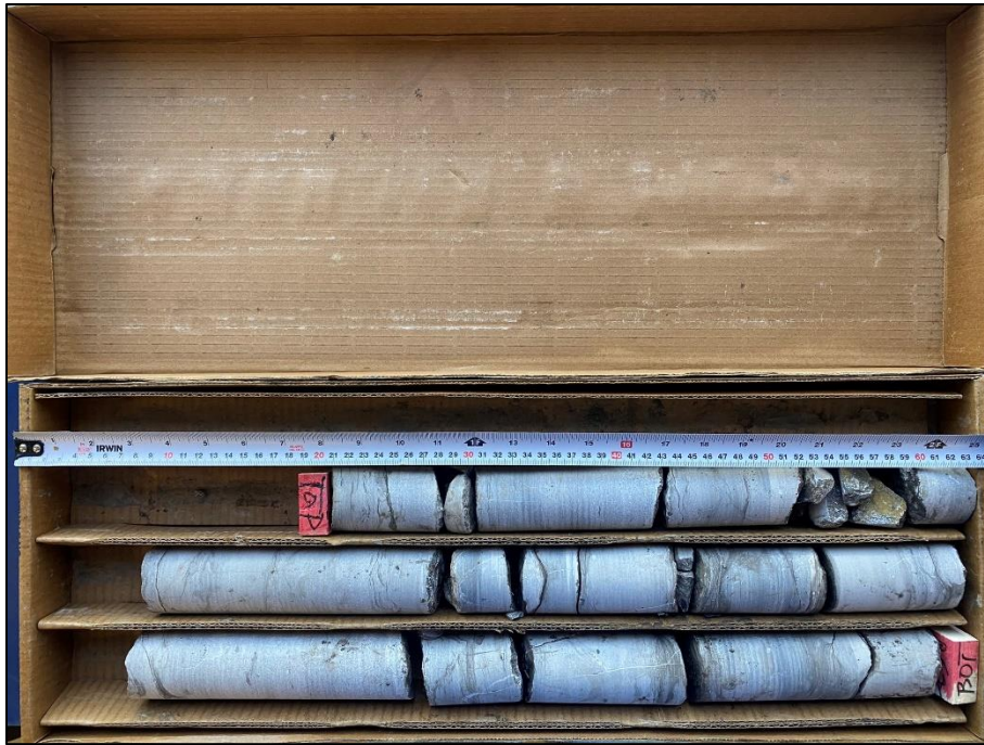
Photo 13: Photograph of RC 2 from BH 2-23 – Depth from 3.18 to 4.67 m – RQD = 76 % and REC = 100 %
