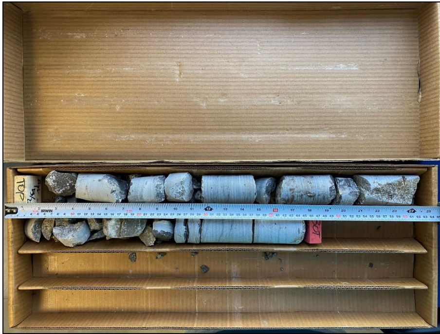
Photo 24: Photograph of RC 2 from BH 4-23 – Depth from 1.63 to 3.12 m – RQD = 59 % and REC = 100 %
