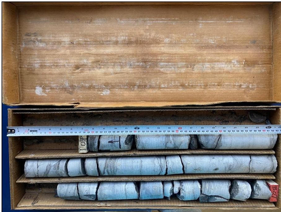
Photo 26: Photograph of RC 4 from BH 4-23 – Depth from 4.62 to 6.12 m – RQD = 64 % and REC = 100 %
