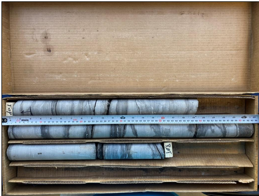
Photo 28: Photograph of RC 6 from BH 4-23 – Depth from 7.62 to 9.12 m – RQD = 97 % and REC = 100 %
