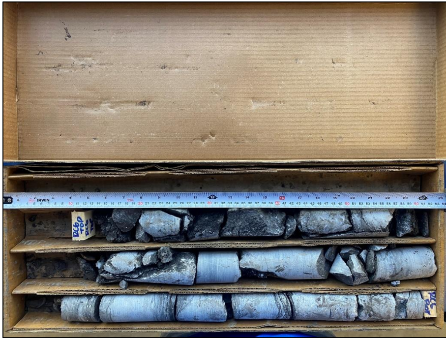
Photo 18: Photograph of RC 7 from BH 2-23 – Depth from 10.67 to 12.17 m – RQD = 93 % and REC = 100 %
