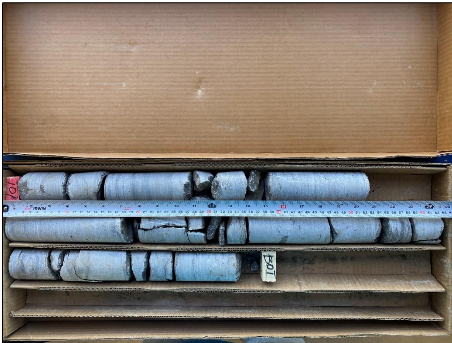
Photo 24: Photograph of RC 2 from BH 4-23 – Depth from 1.63 to 3.12 m – RQD = 59 % and REC = 100 %
