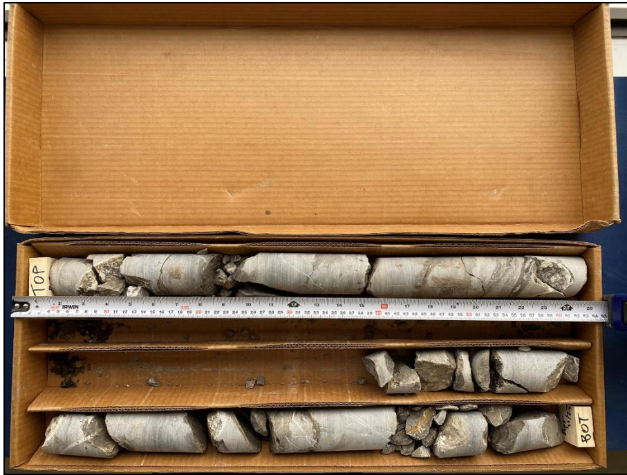
Photo 8: Photograph of RC 8 from BH 1-23 – Depth from 12.14 to 13.64 m – RQD = 56 % and REC = 93 %
