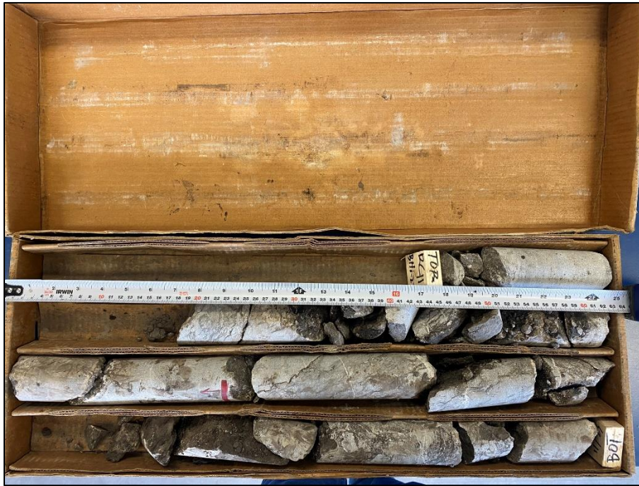
Photo 12: Photograph of RC 1 from BH 2-23 – Depth from 2.51 to 3.18 m – RQD = 62 % and REC = 100 %
