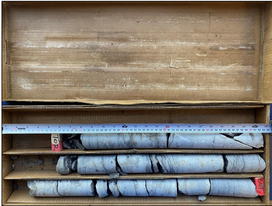
Photo 16: Photograph of RC 5 from BH 2-23 – Depth from 7.67 to 9.17 m – RQD = 59 % and REC = 100 %
