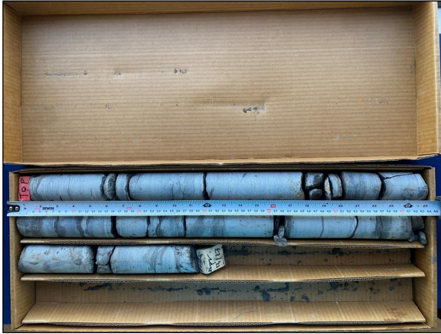
Photo 26: Photograph of RC 4 from BH 4-23 – Depth from 4.62 to 6.12 m – RQD = 64 % and REC = 100 %
