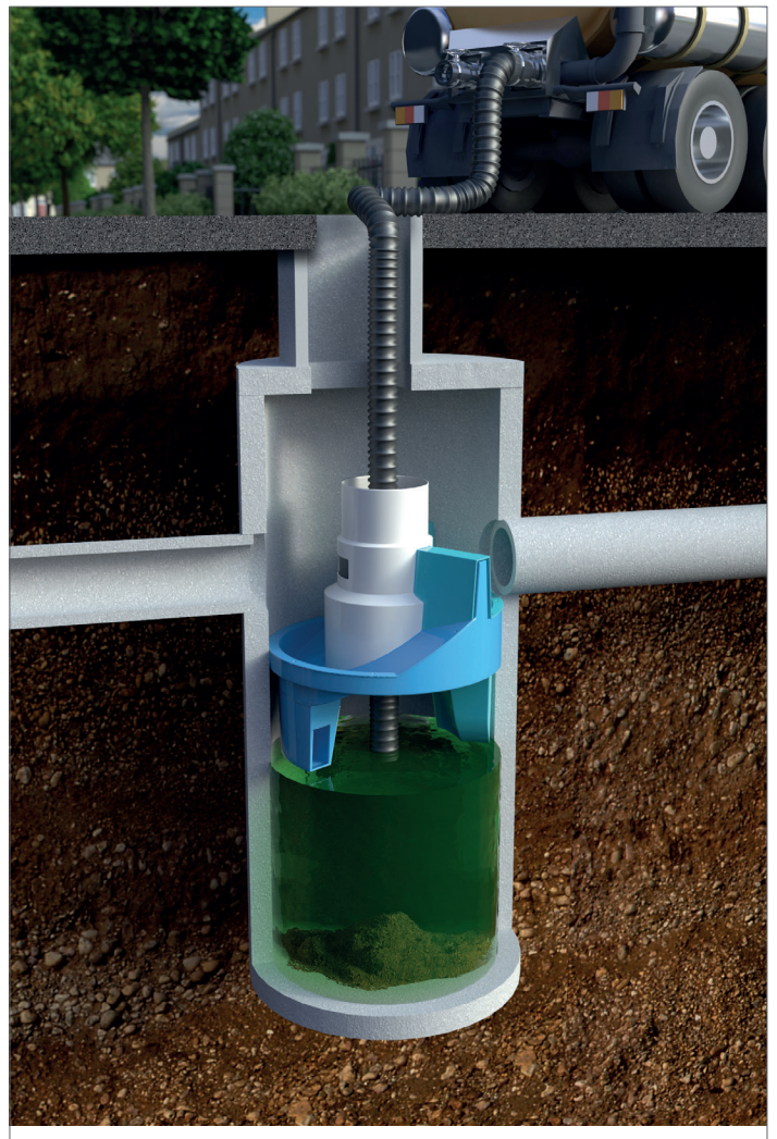
Fig.4 Floatables are removed with a vactor hose
