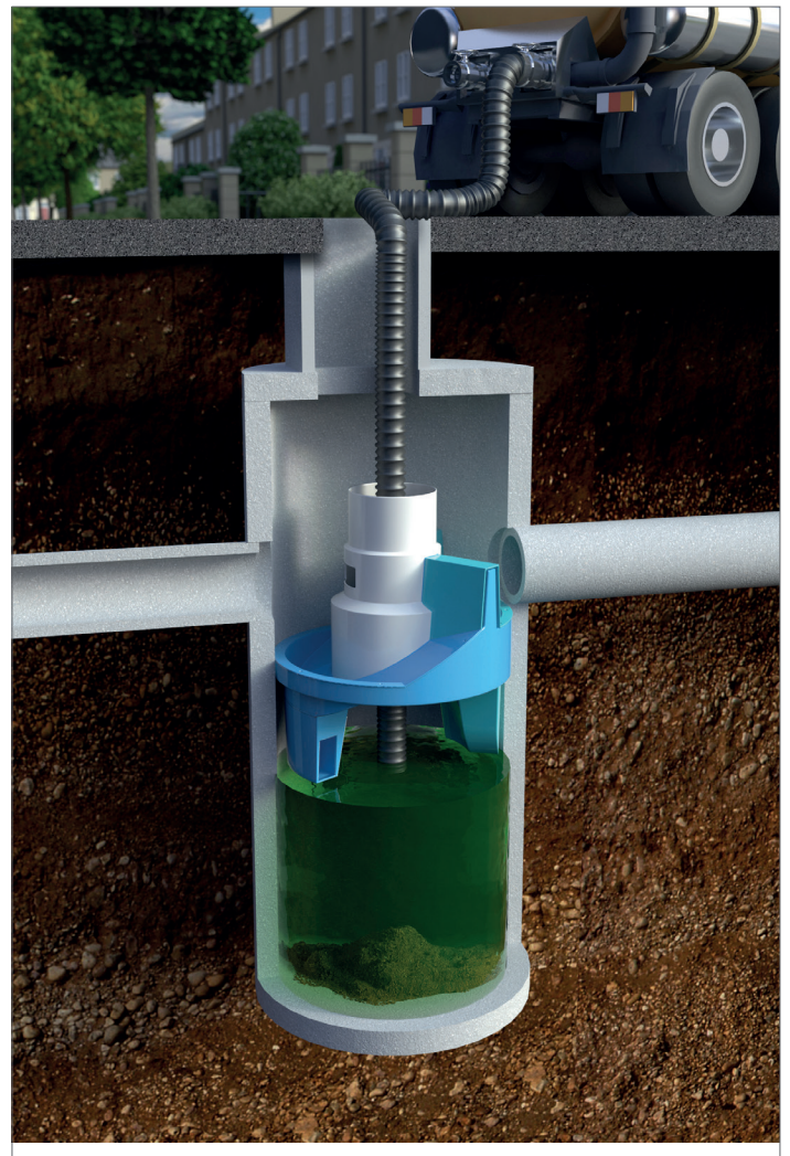
Fig.4 Floatables are removed with a vactor hose
