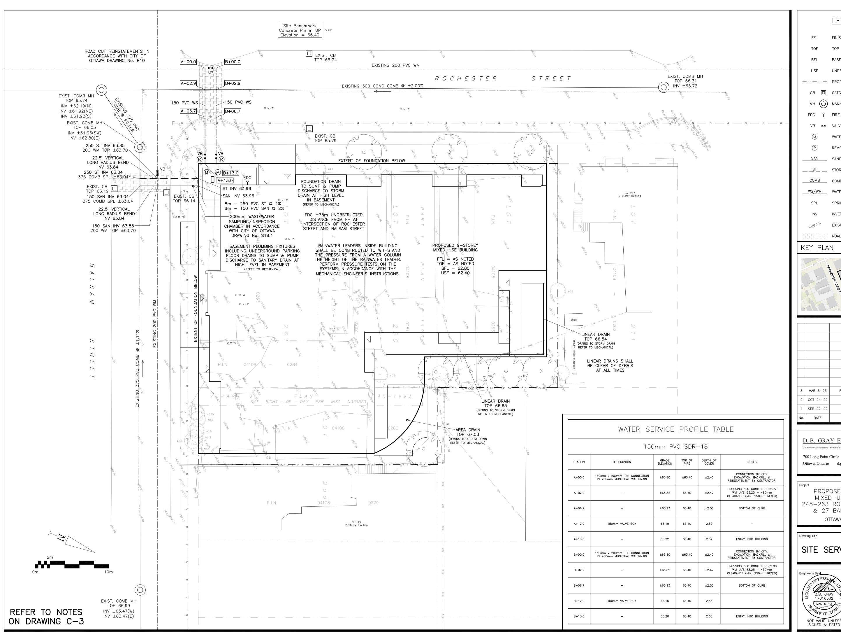
**LEGEND** FINISHED FLOOR ELEVATION TOP OF FOUNDATION BASEMENT FLOOR ELEVATION UNDERSIDE OF FOOTING CB CATCH-BASIN MANHOLE FIRE DEPARTMENT CONNECTION ■ VALVE & VALVE BOX WATER METER REMOTE WATER METER SANITARY SEWER SERVICE \_\_\_\_ST\_\_\_ STORM SEWER SERVICE COMBINED SEWER WS/WM WATER SERVICE/WATERMAIN SPRINGLINE OF PIPE INVERT OF PIPE EXISTING GRADE ELEVATION ROAD CUT REINSTATEMENT KEY PLAN
