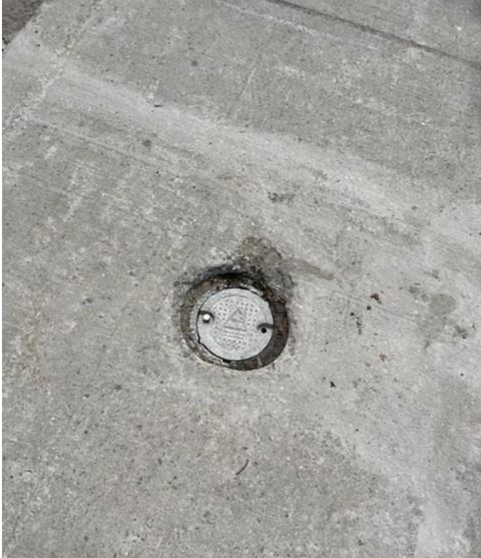
Image 8 – EX-MW6 offsite monitoring well
