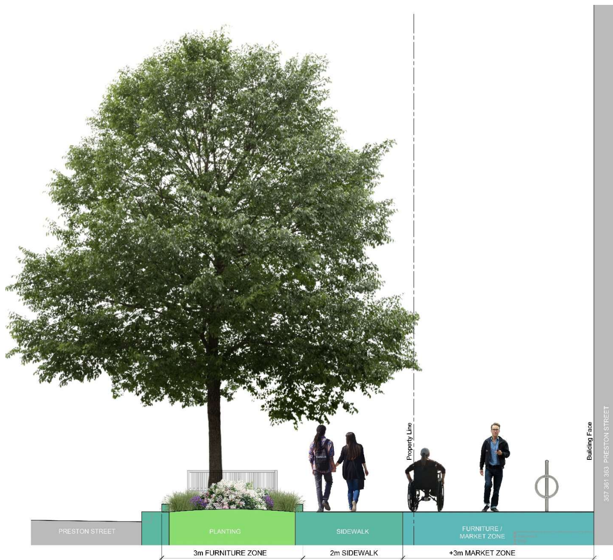
Figure 3: Cross section to illustrate pedestrian realm
