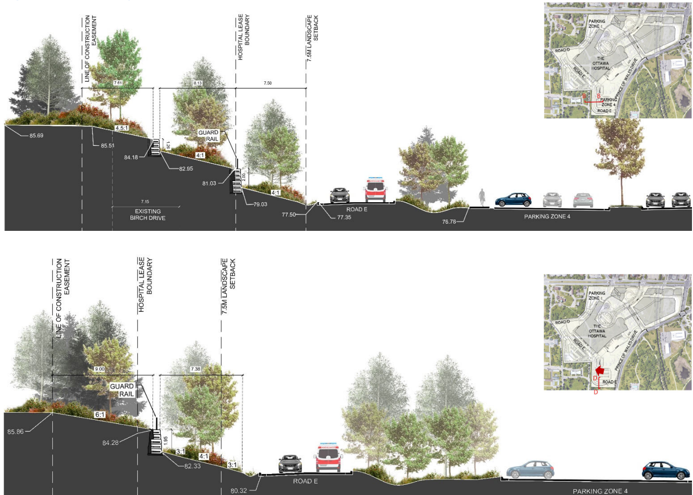
Figure 15: Retaining Wall Sections at Road E
