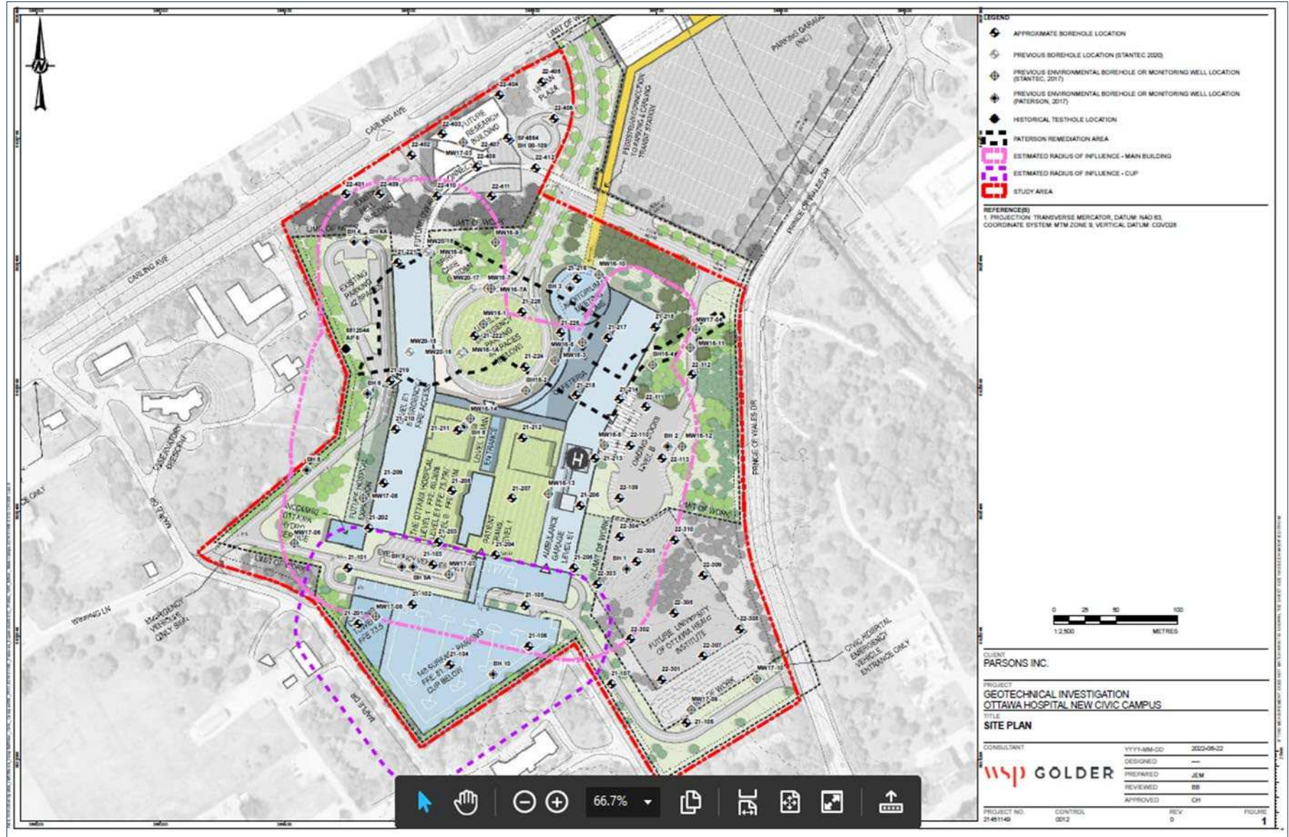
Figure 28: Dewatering Estimated Area of Influence
