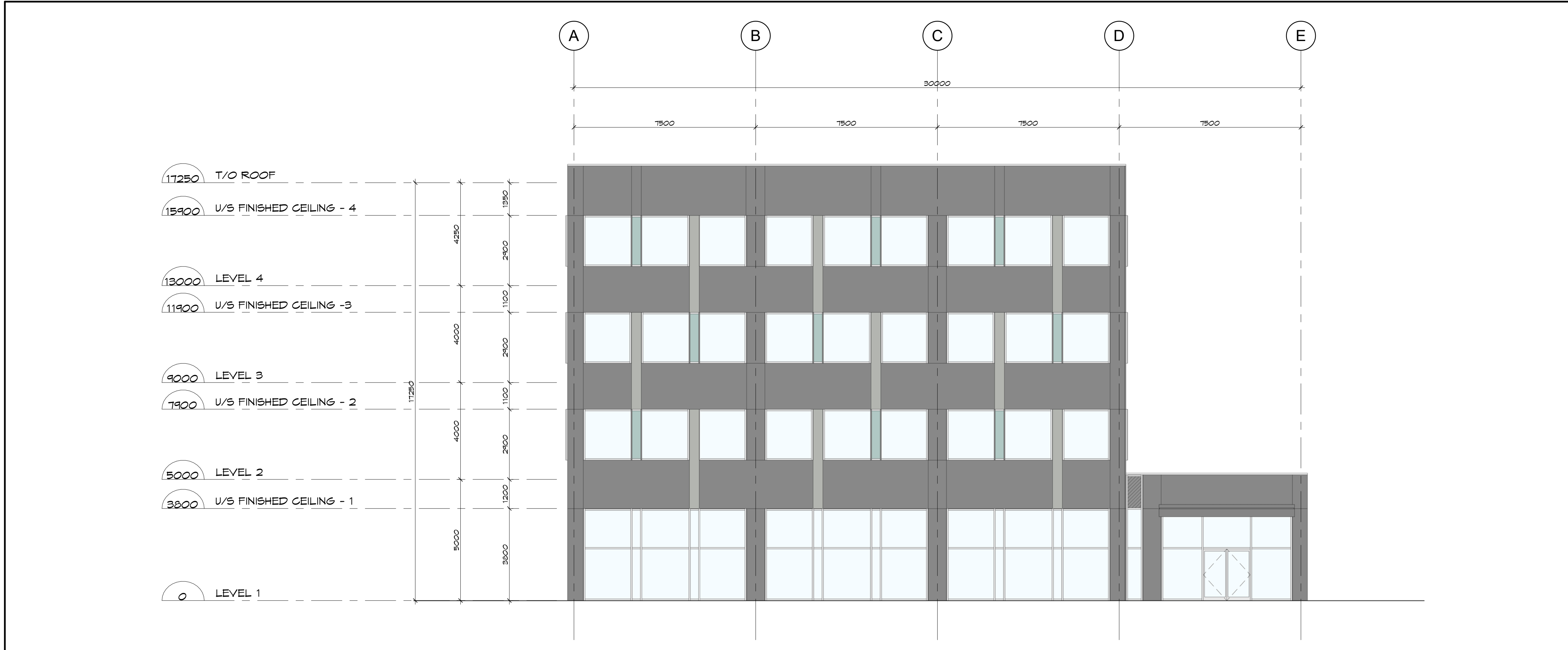
2 ELEVATION @ GRID 6 (facing parking) A-4 SCALE: 1 : 100
