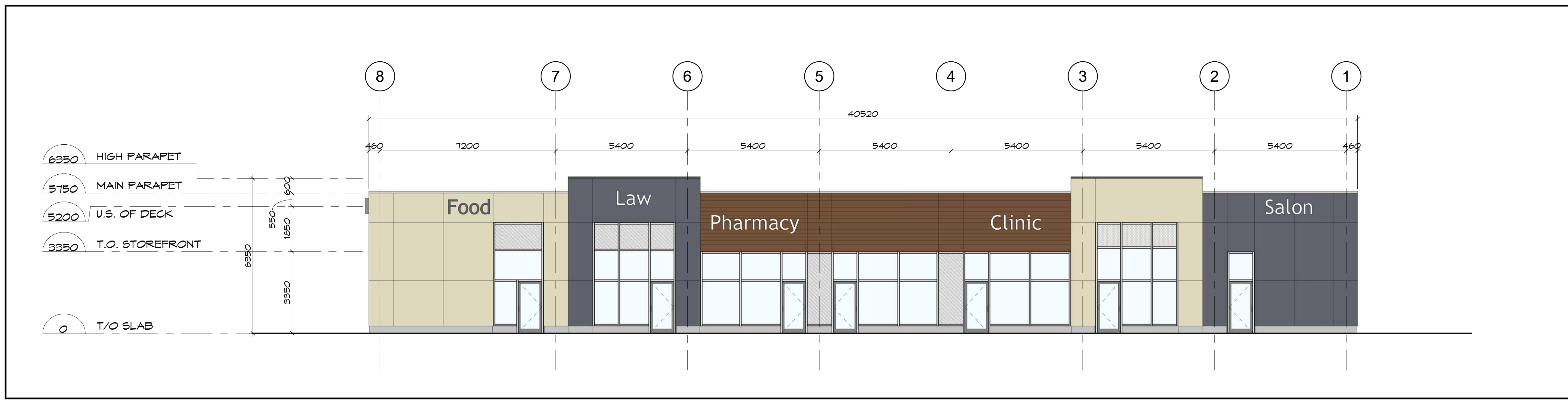
2 ELEVATION @ GRID C (facing street) A-3 SCALE: 1:100
