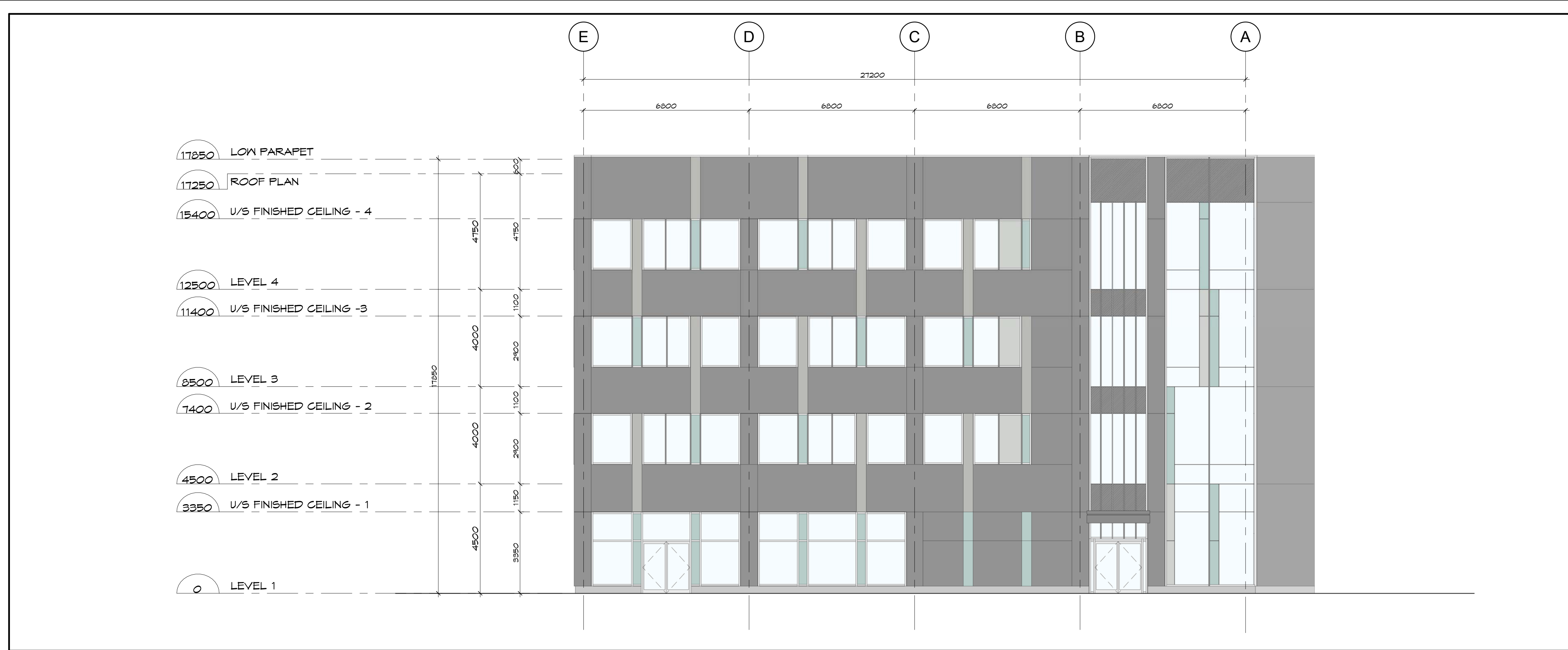
1 WEST ELEVATION @ GRID 1 (facing parking) SCALE: 1 : 100
