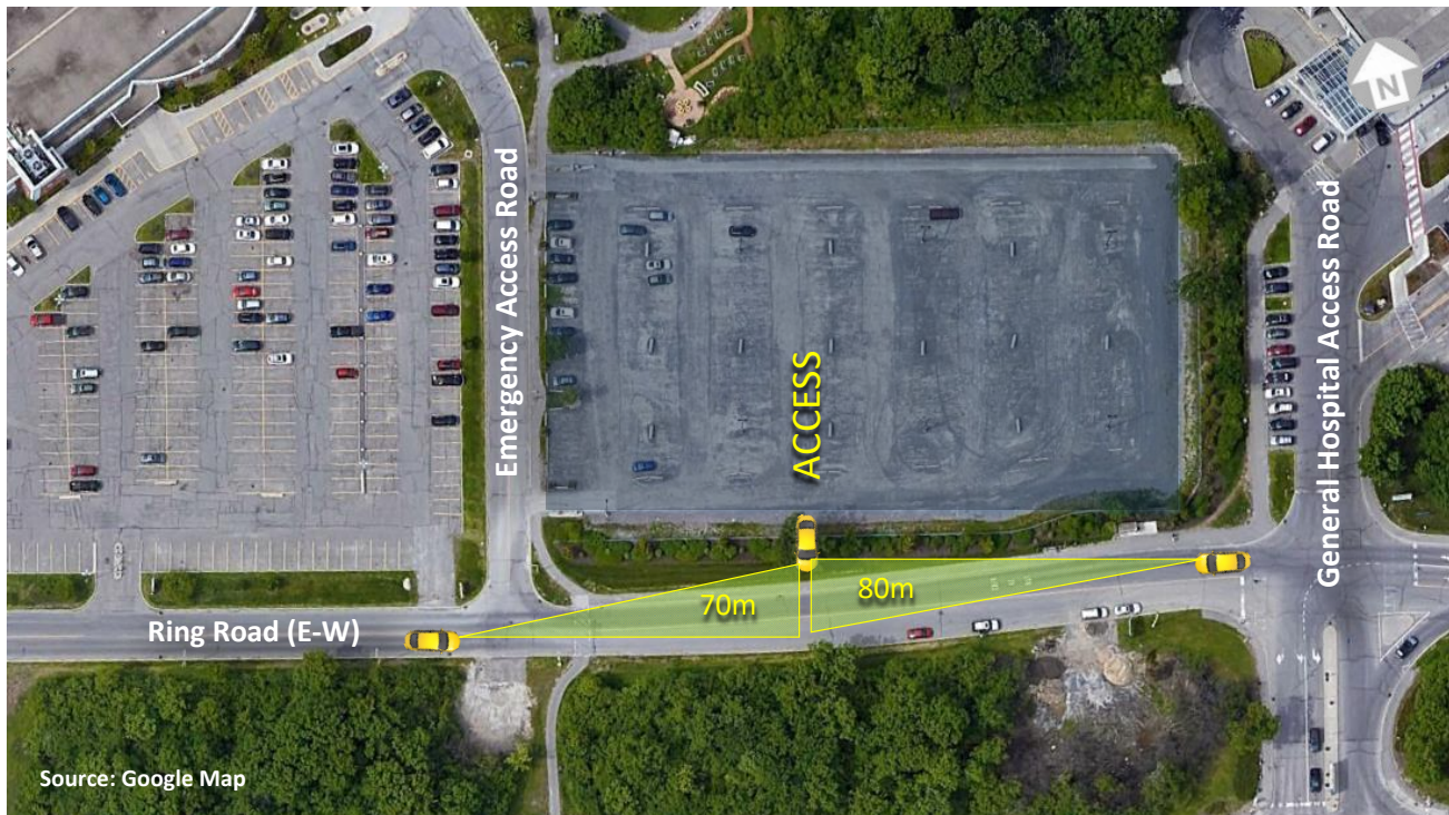
Figure 10: Ring Road (E-W) Access Intersection Sight Distance
