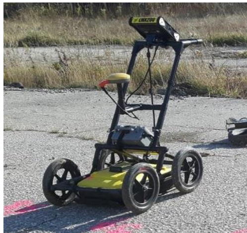
Figure 3-3: Typical GPR 250MHz Smart Cart System Setup
