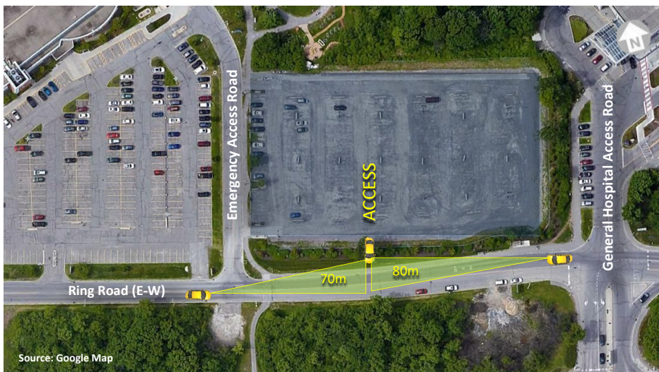
Figure 11: Ring Road (E-W) Access Intersection Sight Distance
