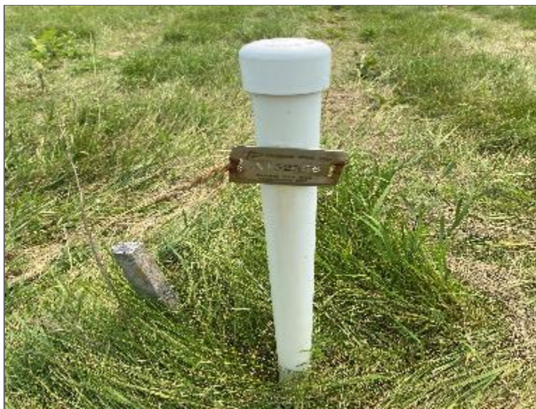
Photo 4 – Typical groundwater monitoring well observed on-Site (installed as part of a previous geotechnical investigation).
