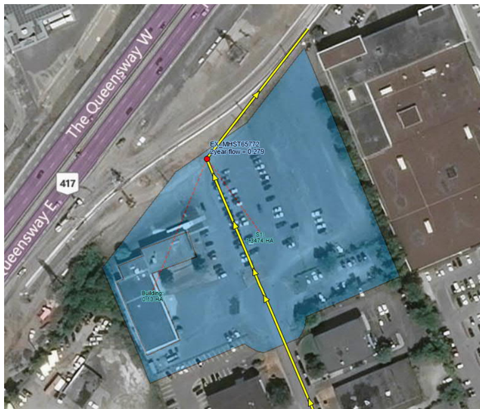
Figure 2: Existing Conditions Catchment Characteristics
