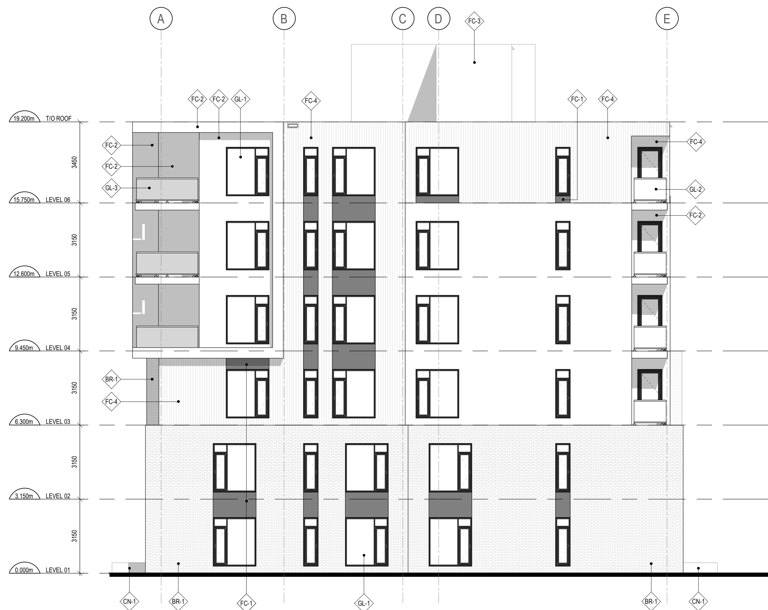
1 WEST BUILDING - WEST ELEVATION A206 SCALE: 1 : 100
