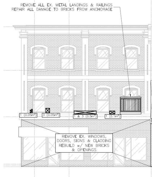
Bank Street removals. Source: Art Engineering,
