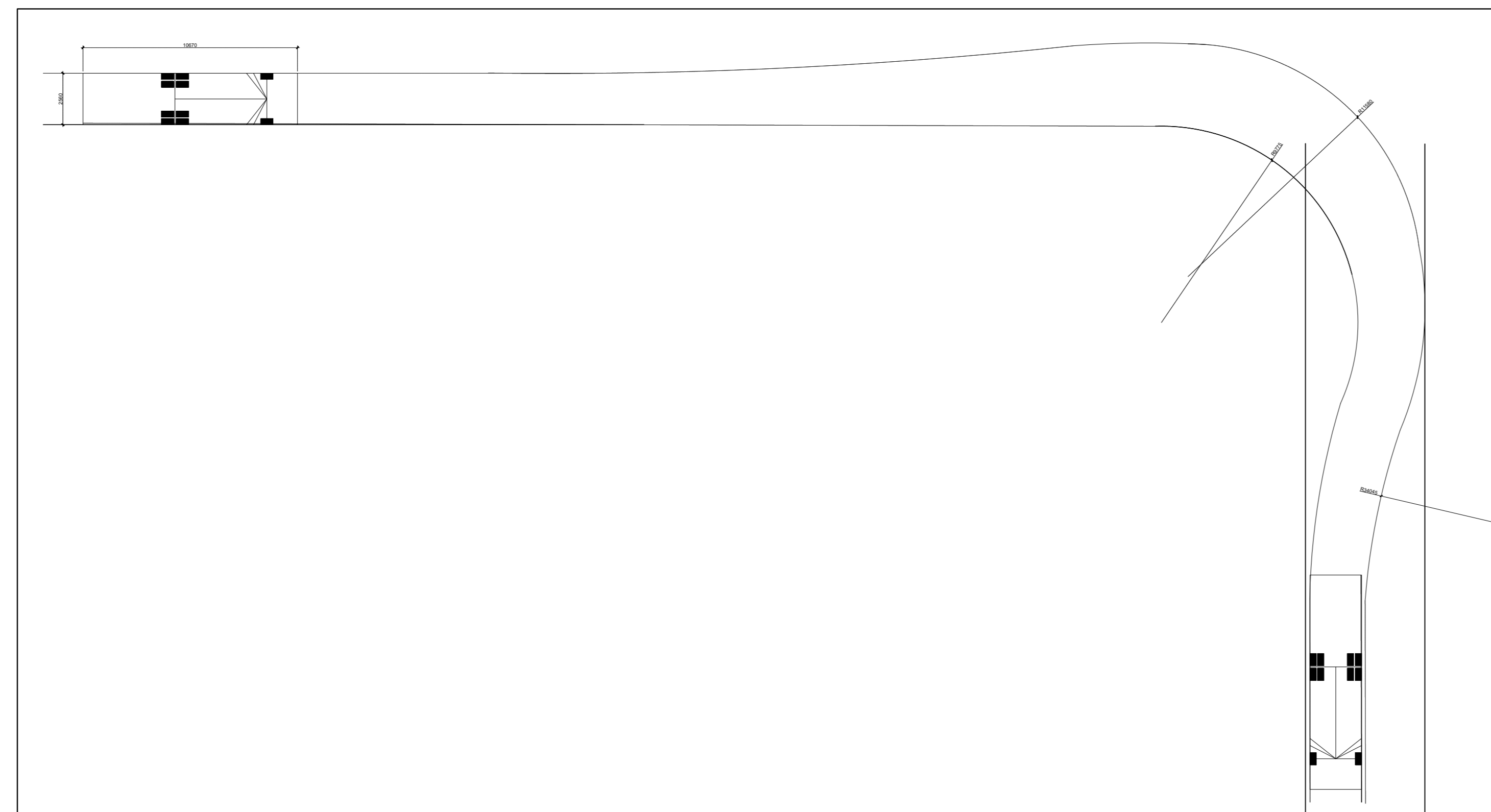
3 GARBAGE TRUCK ROUTE DIMENSIONS SCALE = 1/16" = 1'-0"
