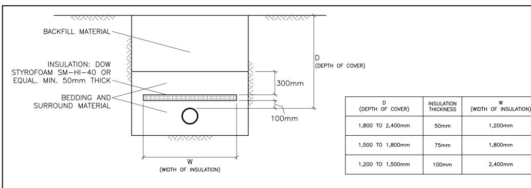
INSULATE WATERMAINS AND WATER SERVICES AS INDICATED AND WHERE DEPTH OF COVER IS LESS THAN 2,400mm.
