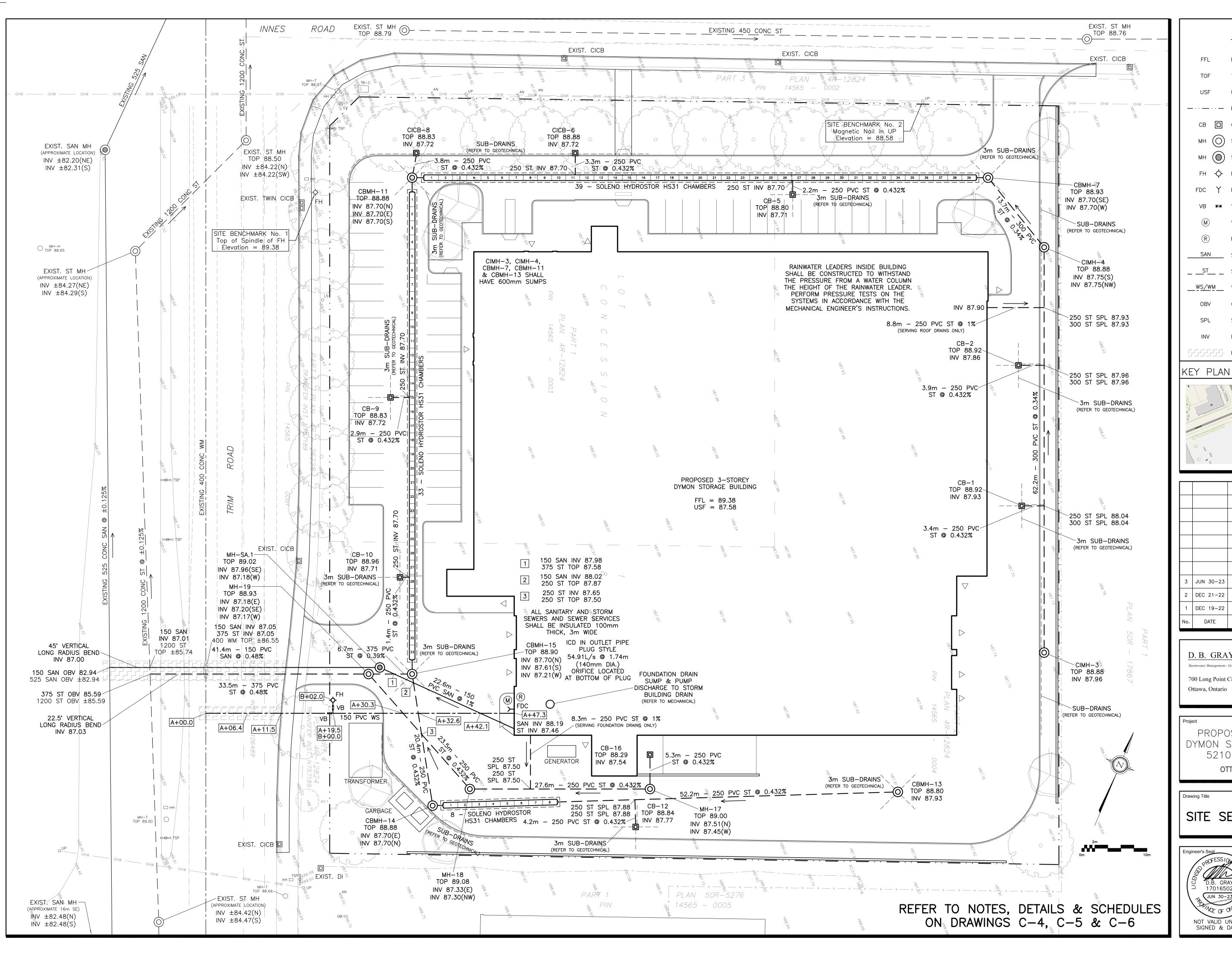
**LEGEND** FINISHED FLOOR ELEVATION TOP OF FOUNDATION UNDERSIDE OF FOOTING - · · - PROPERTY LINE CB CATCH-BASIN STORM MANHOLE ( SANITARY MANHOLE FH -O- FIRE HYDRANT FDC Y FIRE DEPARTMENT CONNECTION VALVE & VALVE BOX WATER METER REMOTE WATER METER SANITARY SEWER \_ \_ST\_ \_ STORM SEWER <u>WS/WM</u> WATER SERVICE/WATERMAIN OBVERT OF PIPE SPRINGLINE OF PIPE INVERT OF PIPE ROAD CUT REINSTATEMENT
