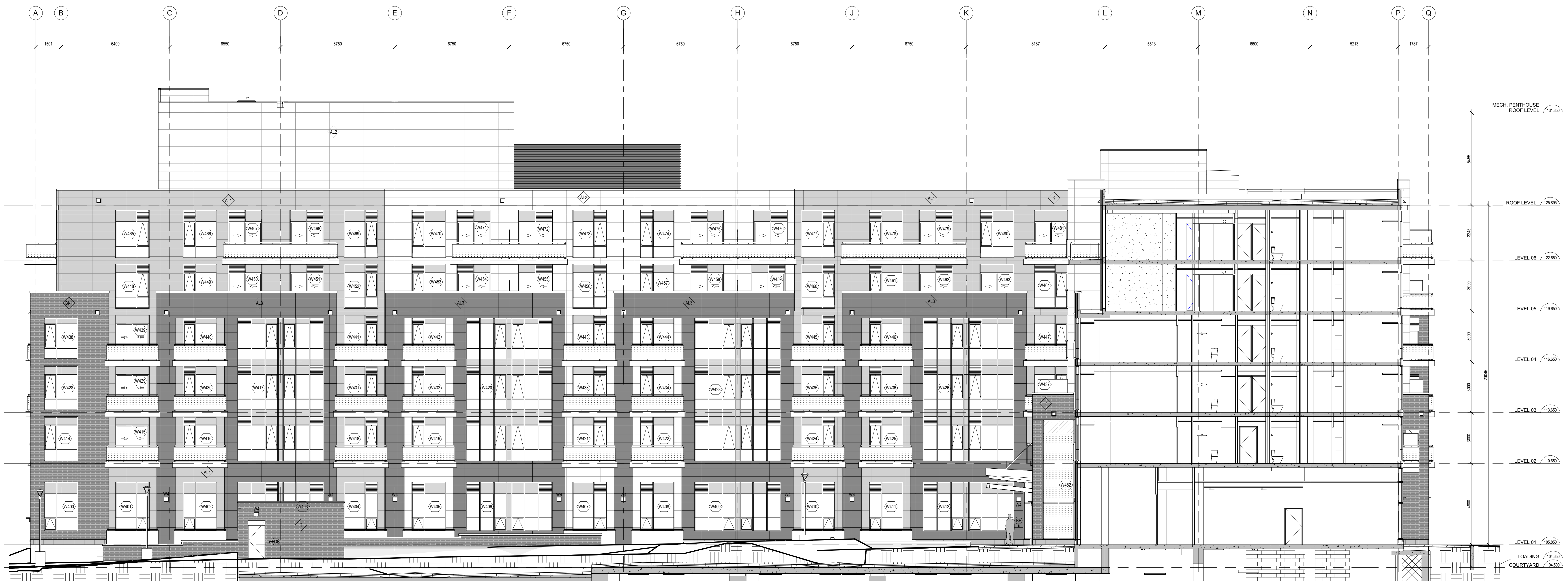
2 SOUTH BUILDING ELEVATION - PHASE 2 A-201A SCALE 1 : 100
