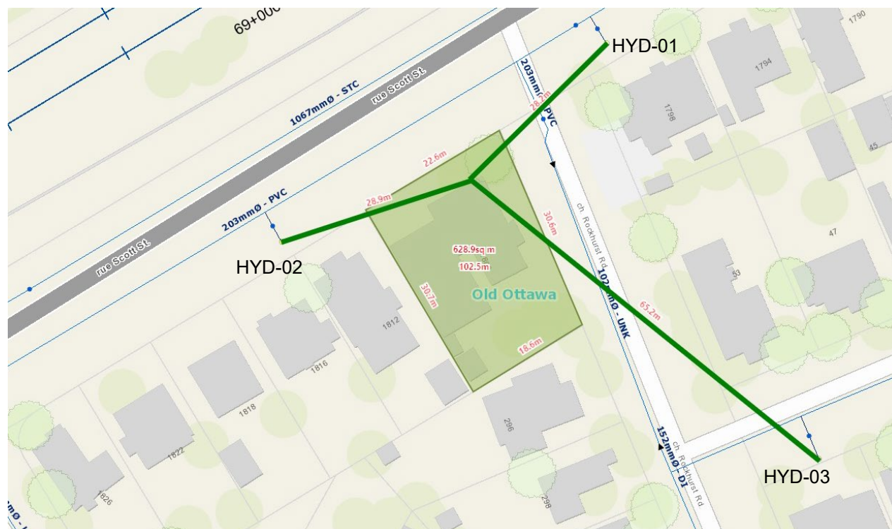
Figure 2: Fire Hydrant Coverage Sketch
