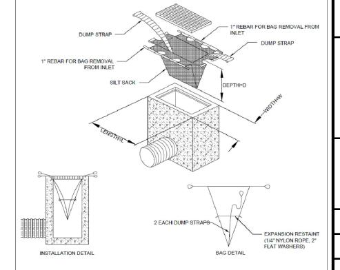
INLET SEDIMENT CONTROL DEVICE
