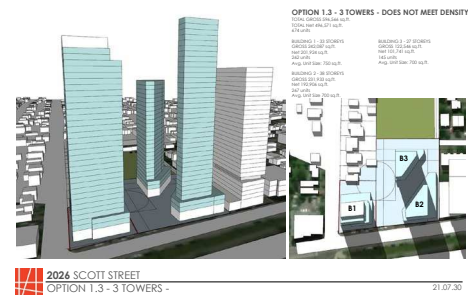
2026 SCOTT STREET OPTION 1.3 - 3 TOWERS - DOES NOT MEET DENSITY 21.07.30 Fig. 38.0 Alternative Massing Study.
