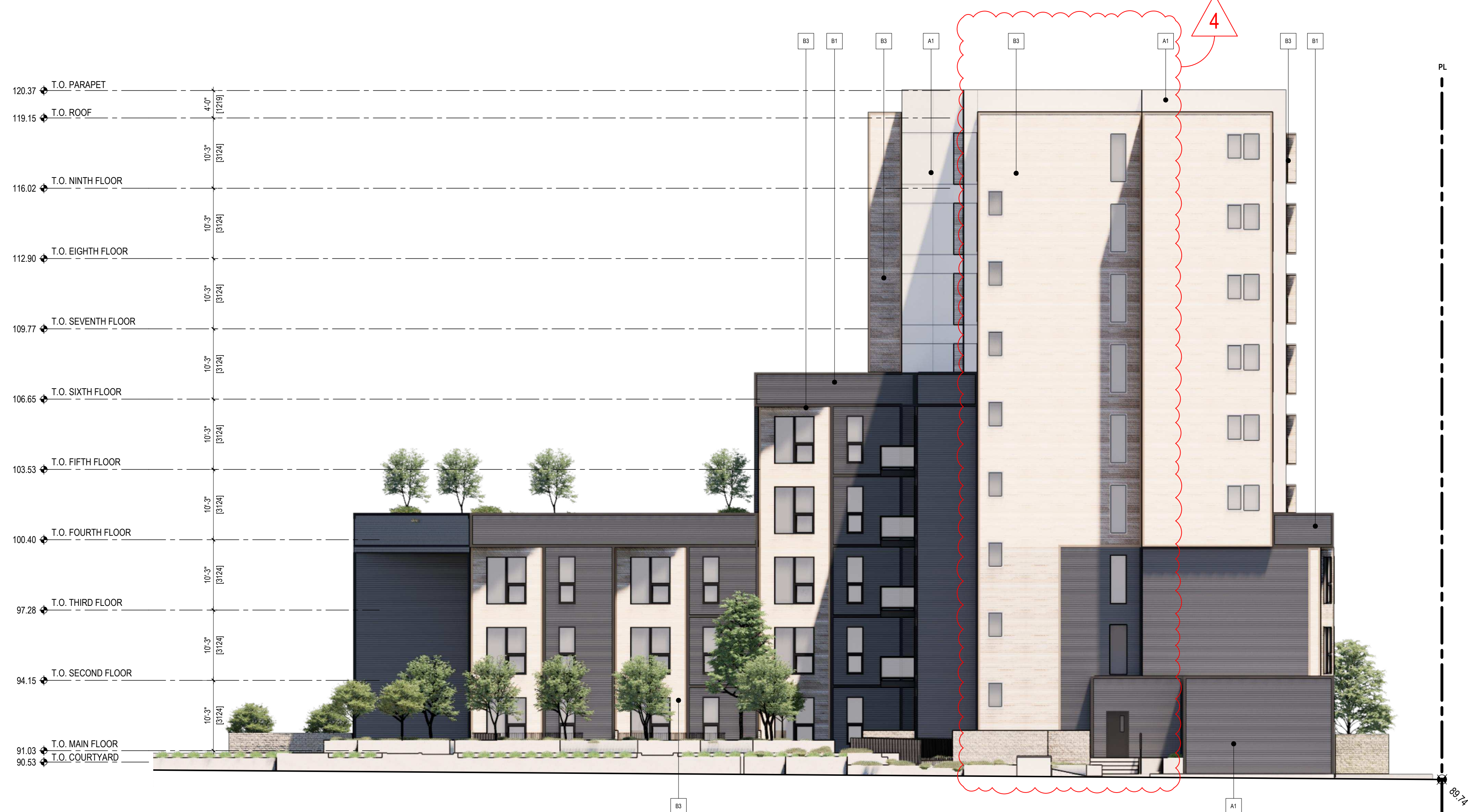
1 BUILDING B - WEST ELEVATION DP.303 3/32" - 1'-0"
