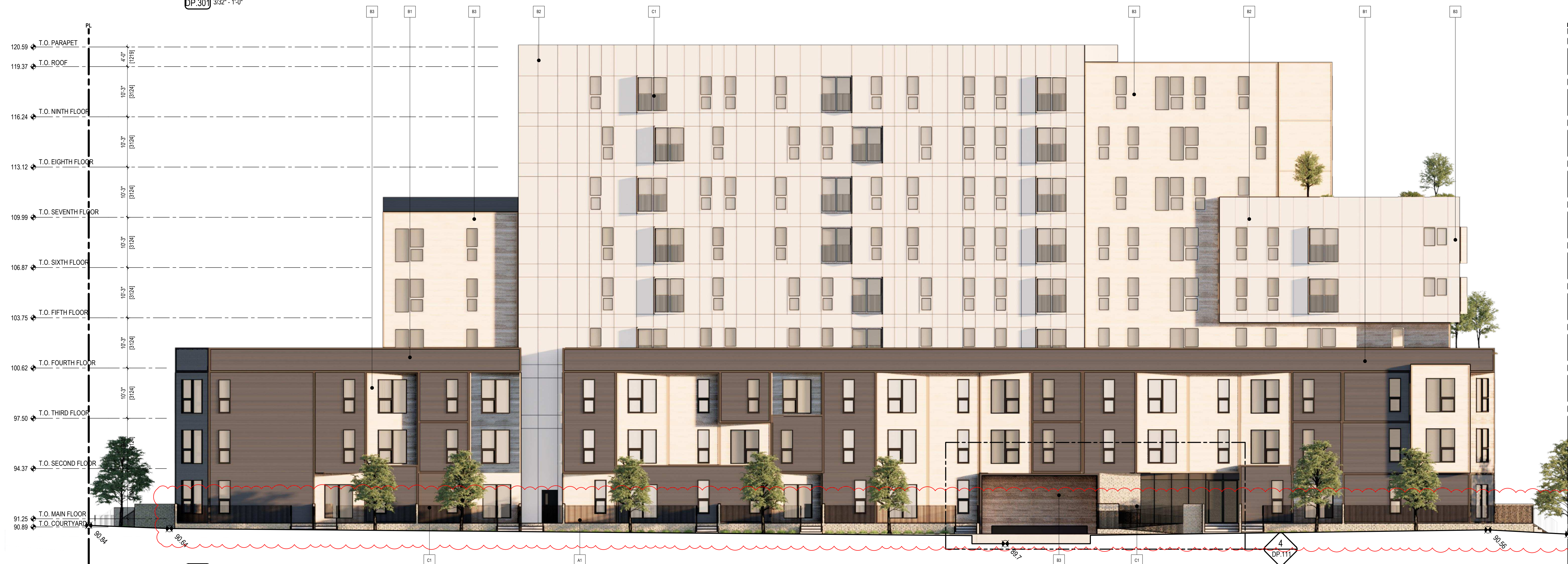
2 BUILDING A - NORTH ELEVATION DP.301 3/32" - 1'-0"
