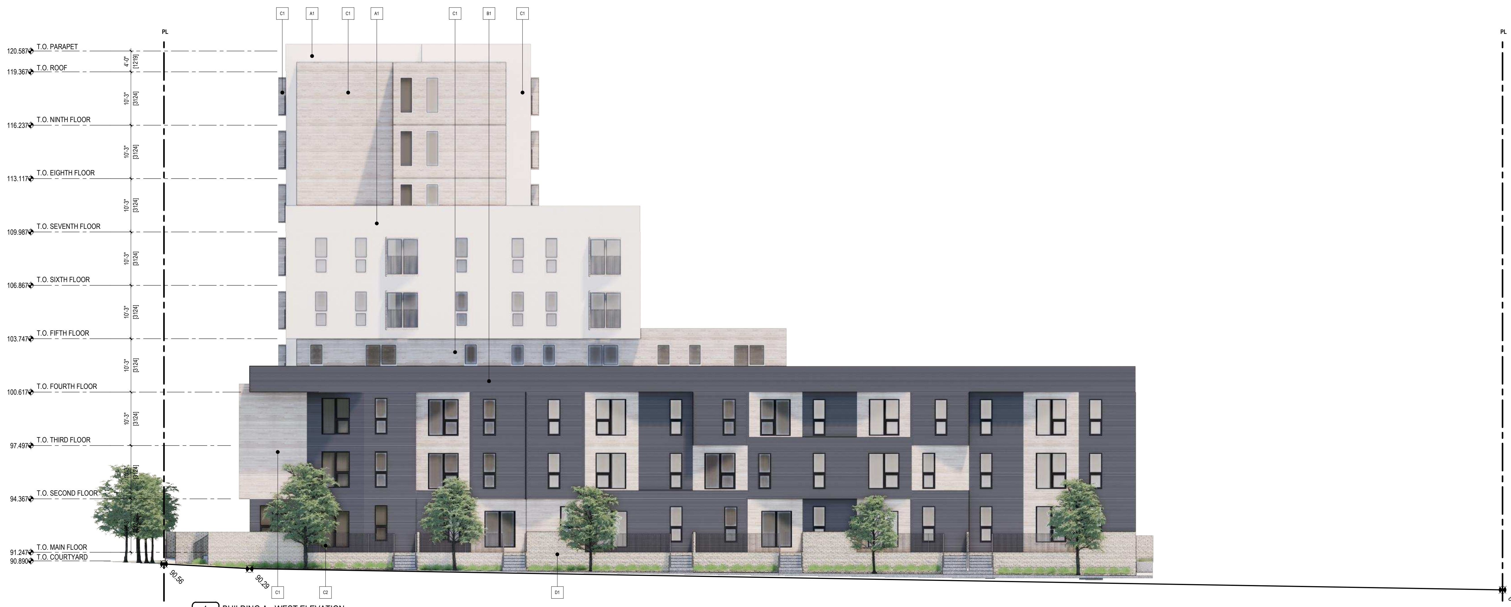
1 BUILDING A - WEST ELEVATION DP.301 3/32" - 1'-0"
