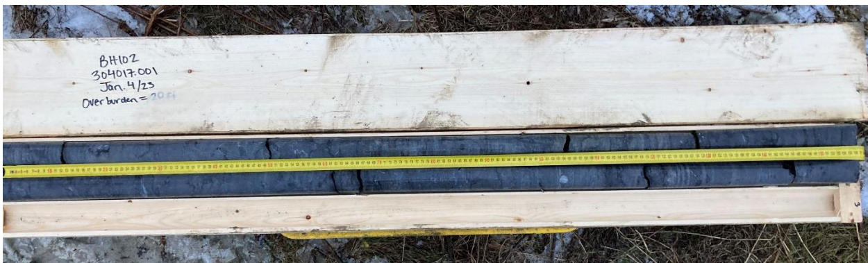
Photo 2 – Borehole BH102, Rock Core
