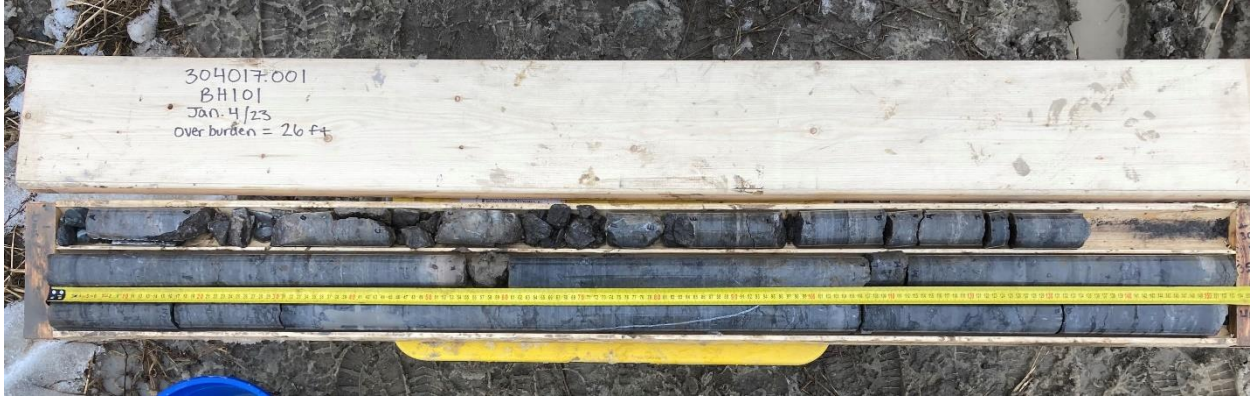
Photo 1 – Borehole BH101, Rock Core
