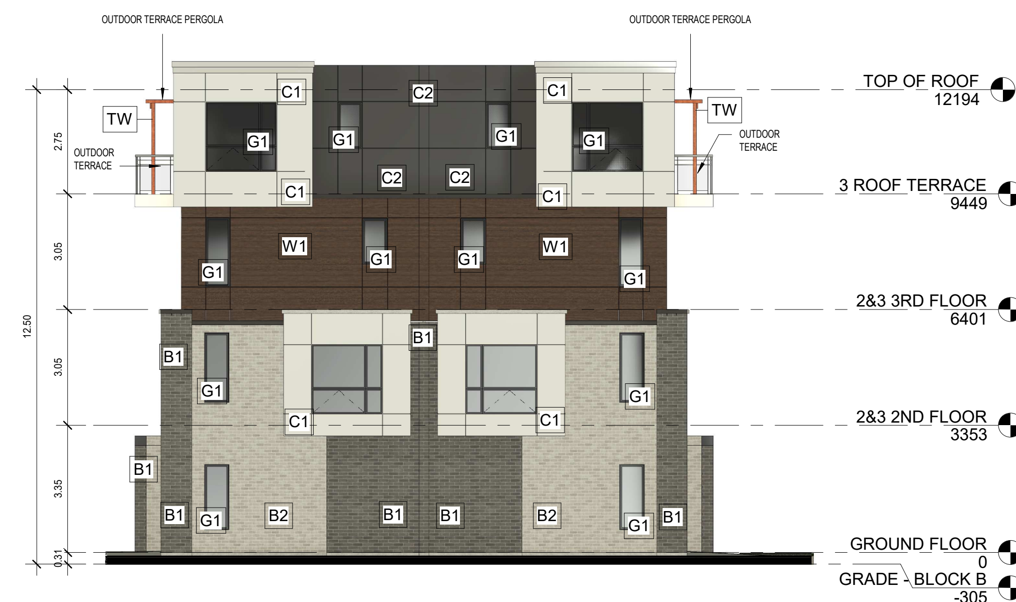
3 SPA - BLOCK B - WEST ELEVATION 1 : 100
