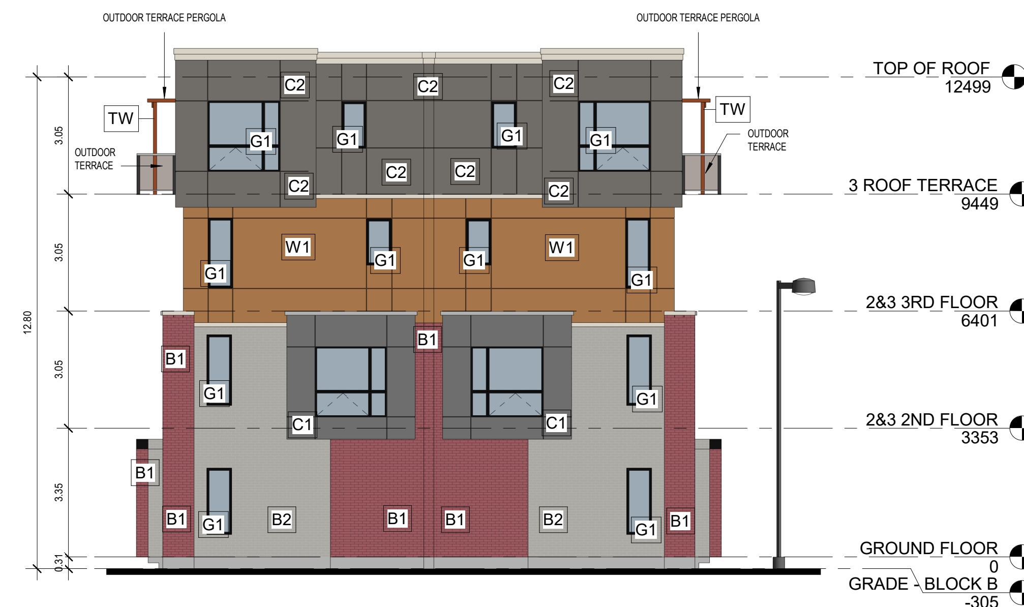
3 SPA - BLOCK B - WEST ELEVATION
