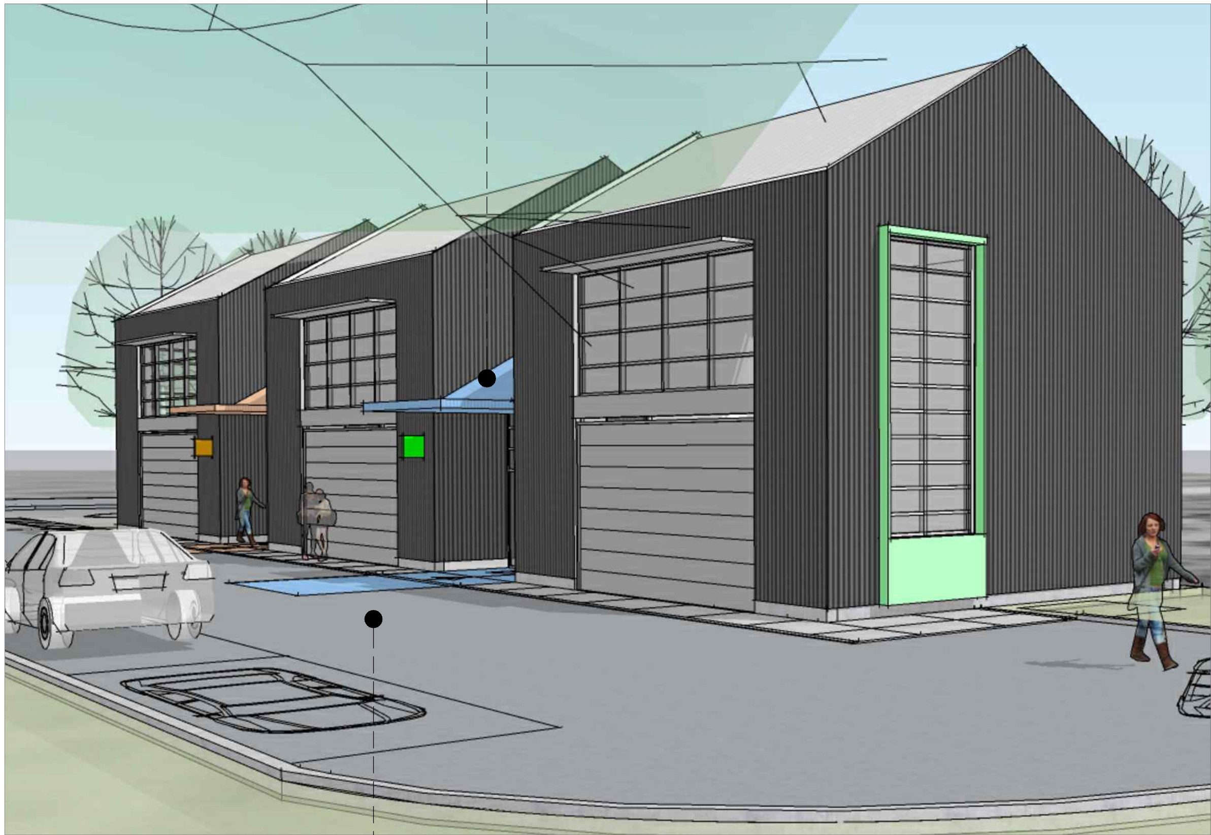
PAVERS - in roadway to visually identify entrances
