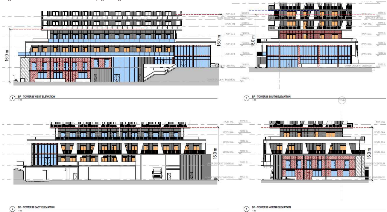
Figure 42. Tower B - Bird friendly glazing and treatment
