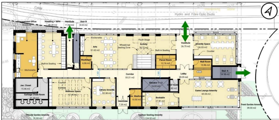
Figure 4: Proposed Main Floor (Source: Diamond Schmitt Architects)
