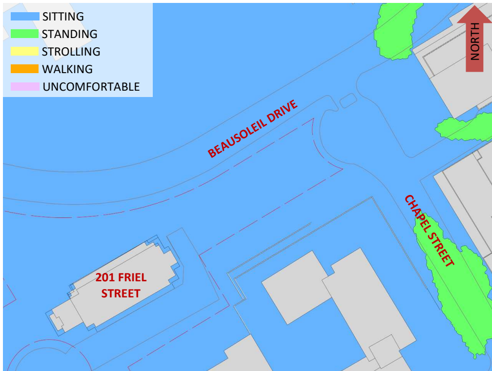
FIGURE 4B: SUMMER – WIND COMFORT, GRADE LEVEL – EXISTING MASSING
