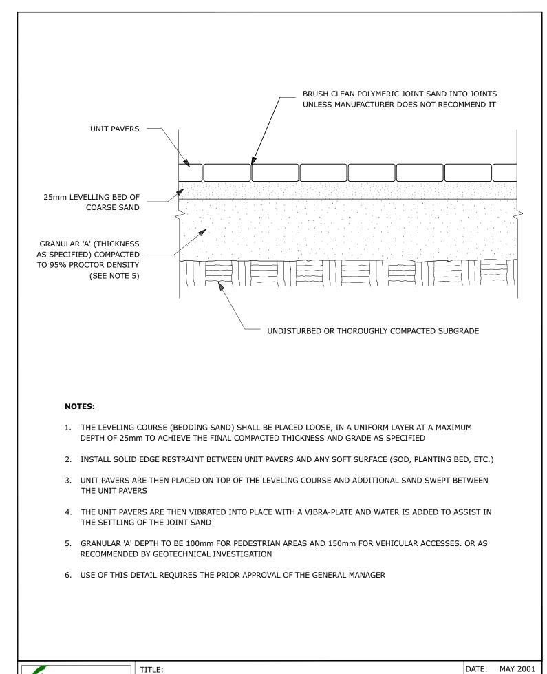
UNIT PAVING - ON GRANULAR BASE
