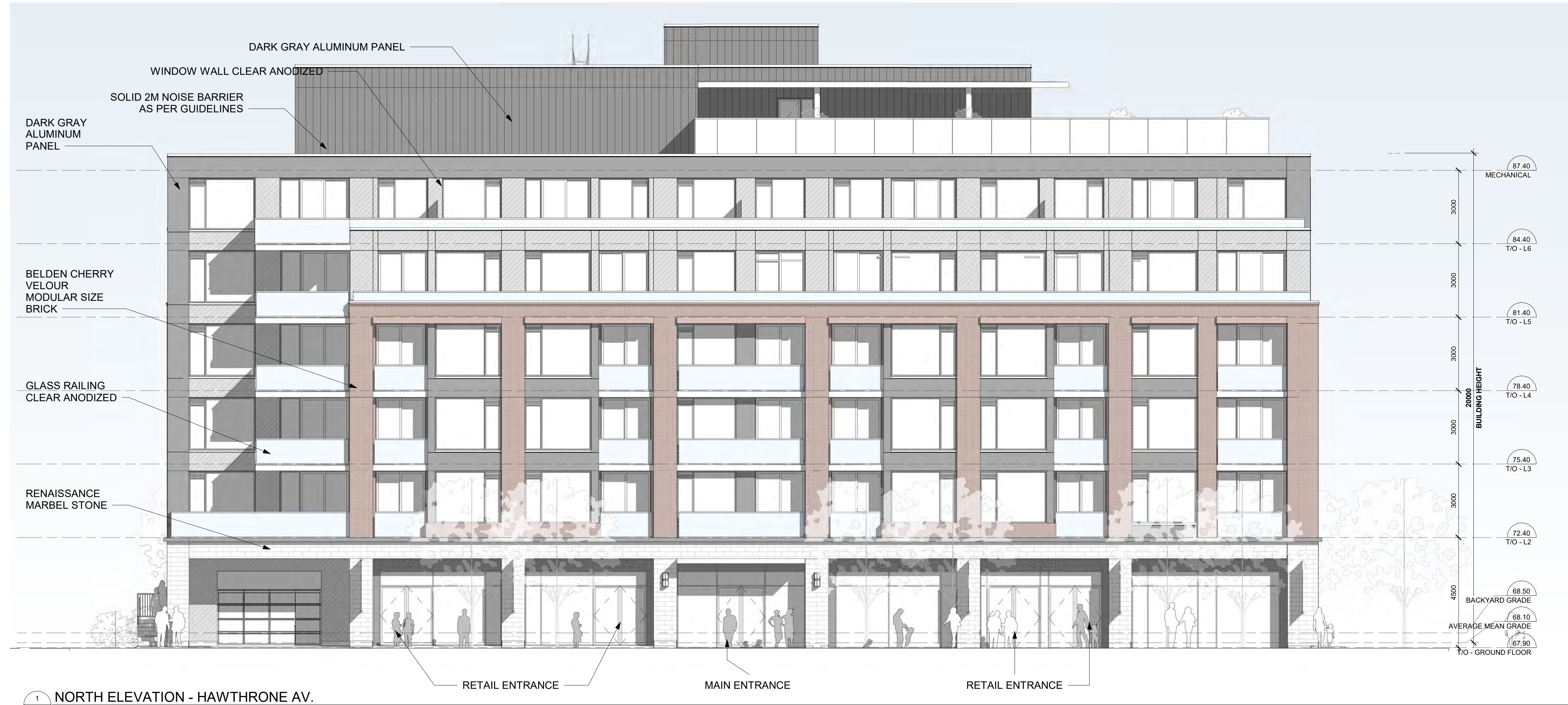
1 NORTH ELEVATION - HAWTHORNE AV. A-103 1 : 100
