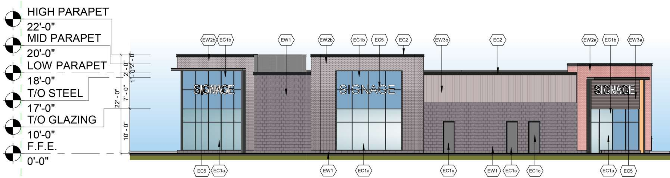
7 BUILDING B - NORTH-EAST ELEVATION A302 1 : 150
