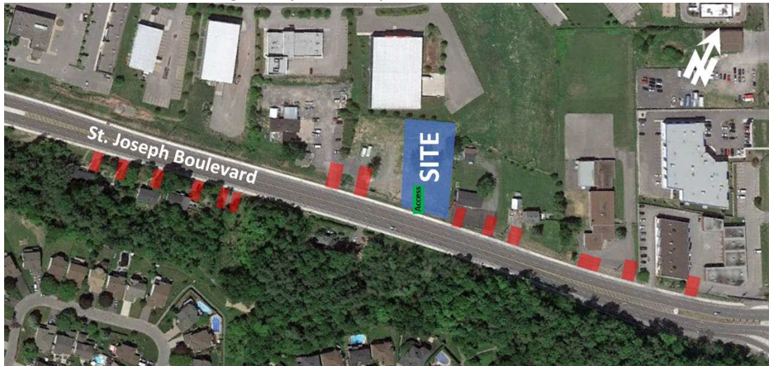
Figure 3: Adjacent Driveways within 200m of Site Access
