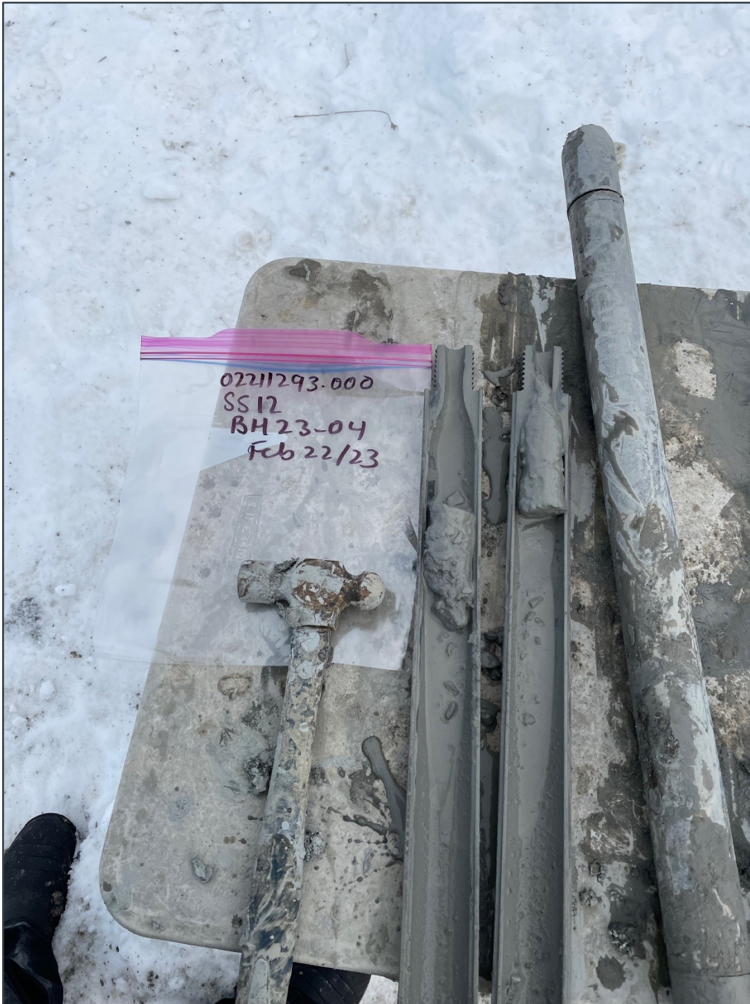
Site Photograph 2. Overview of split spoon sampling (February 22, 2023).
