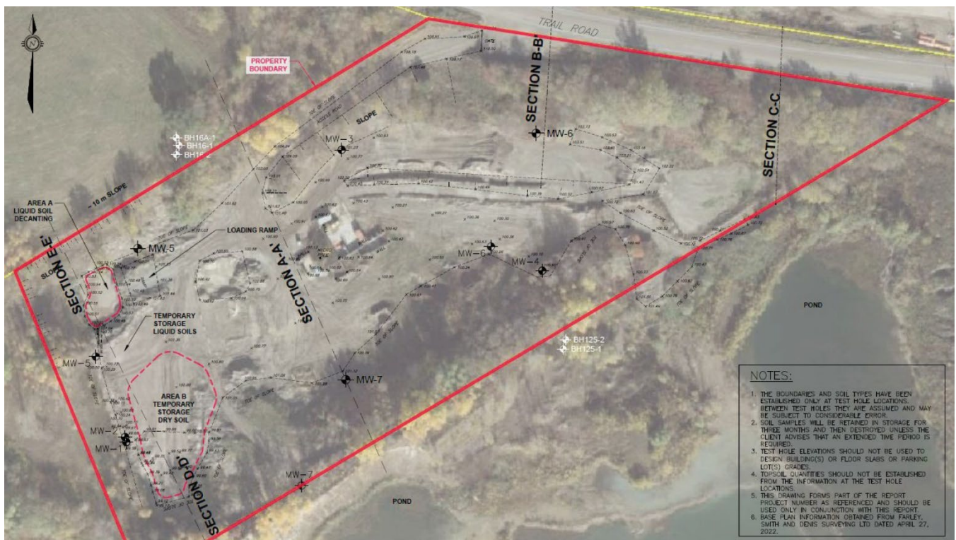
Figure 5: Site Plan identifying soil storage areas on site, as well as grading, and monitoring well locations.
