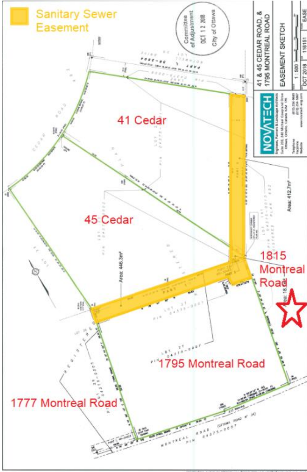
Figure 5: Sanitary sewer easement highlighted, approved by Committee of Adjustment Decisions D08-01-18/B-00369; D08-01-18/B-00370; D08-01-18/B-00368.
