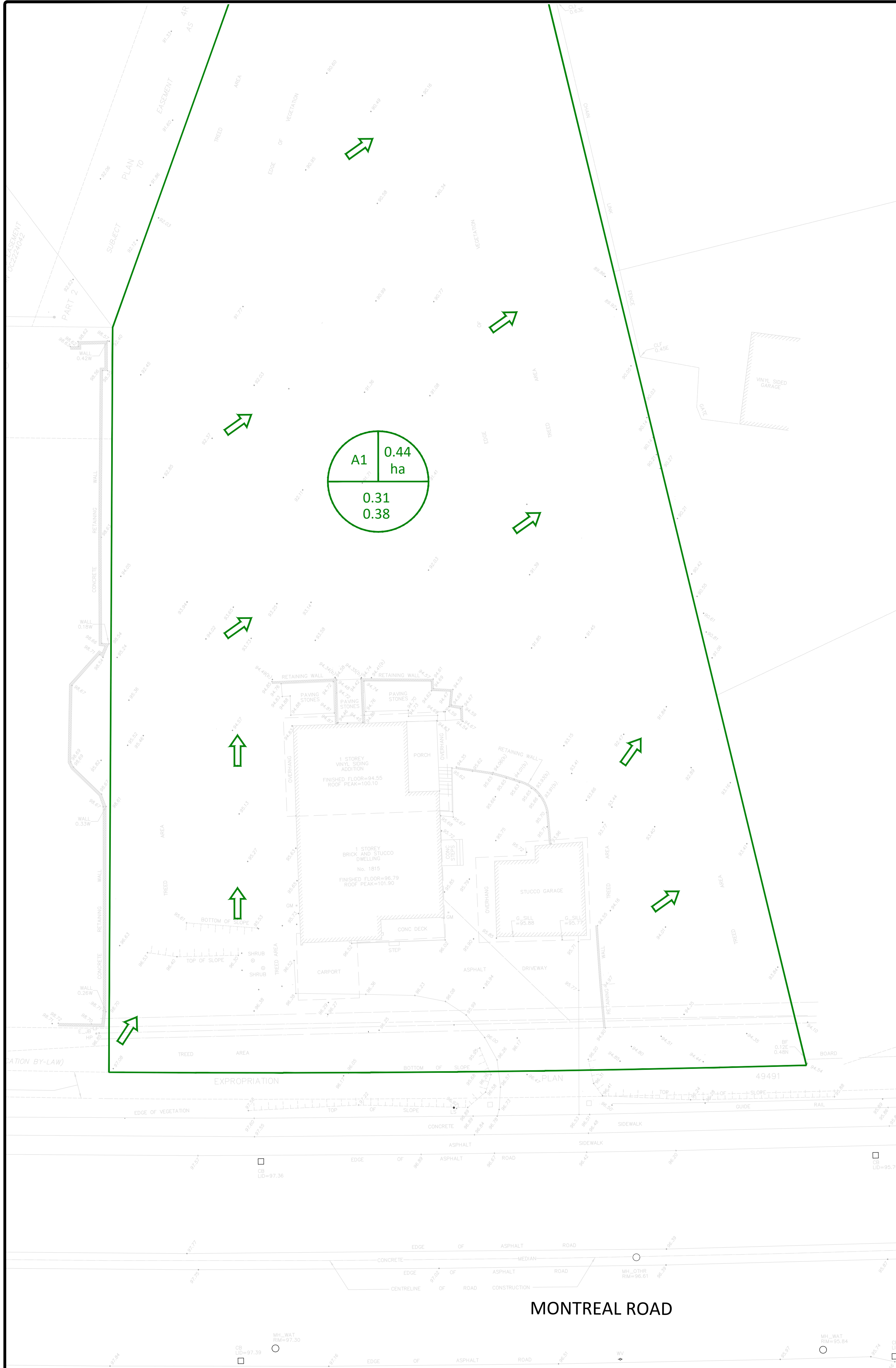
1 PRE-DEVELOPMENT DRAINAGE AREA PLAN 1:200
