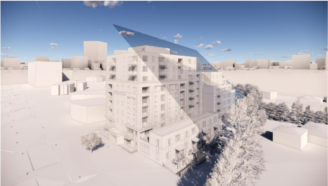
Figure 21: Architectural Perspectives showing the application of a 45-degree angular plane from the East.
