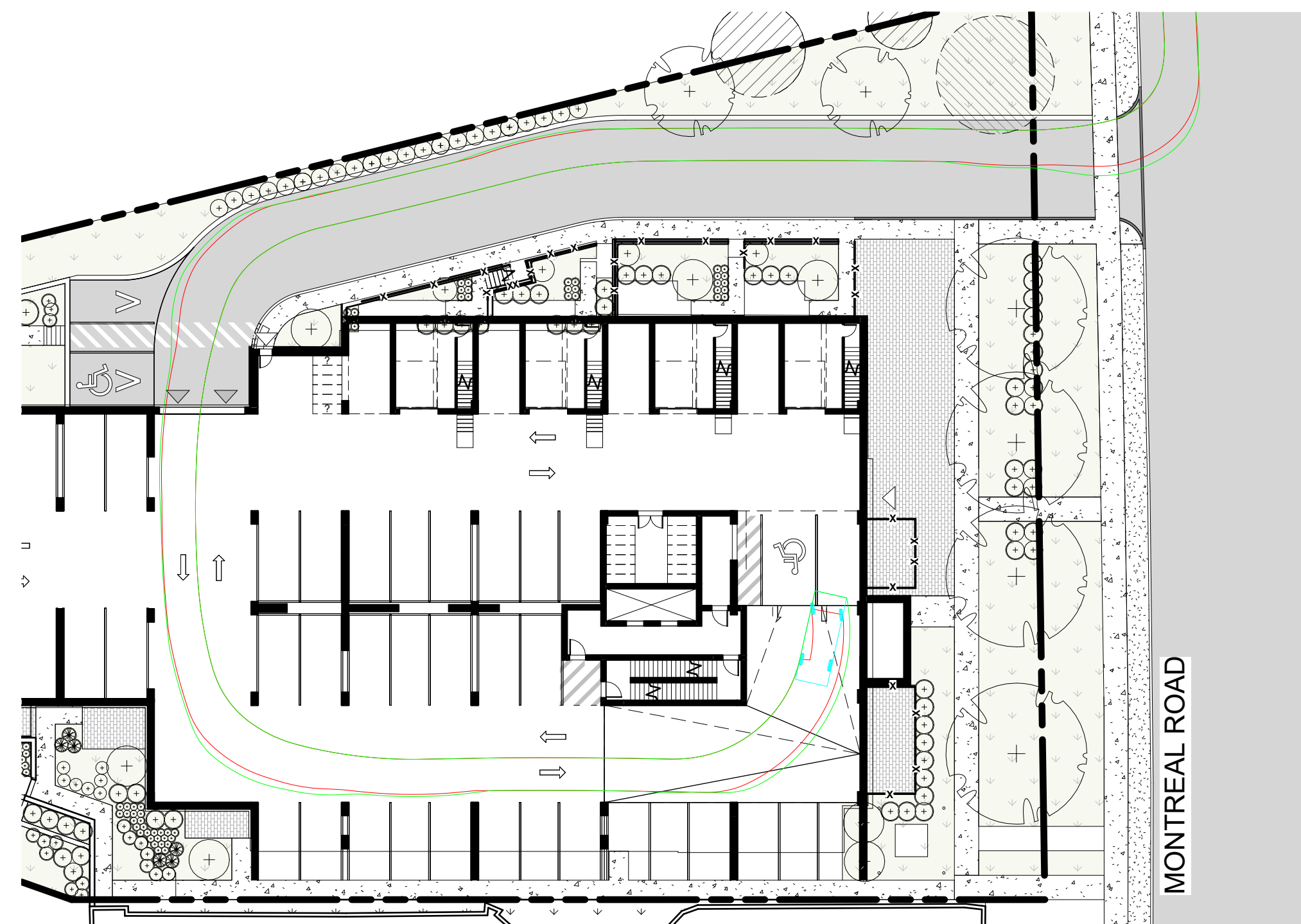
1 TURNING TEMPLATE - Car Entering A102 | 1:300
