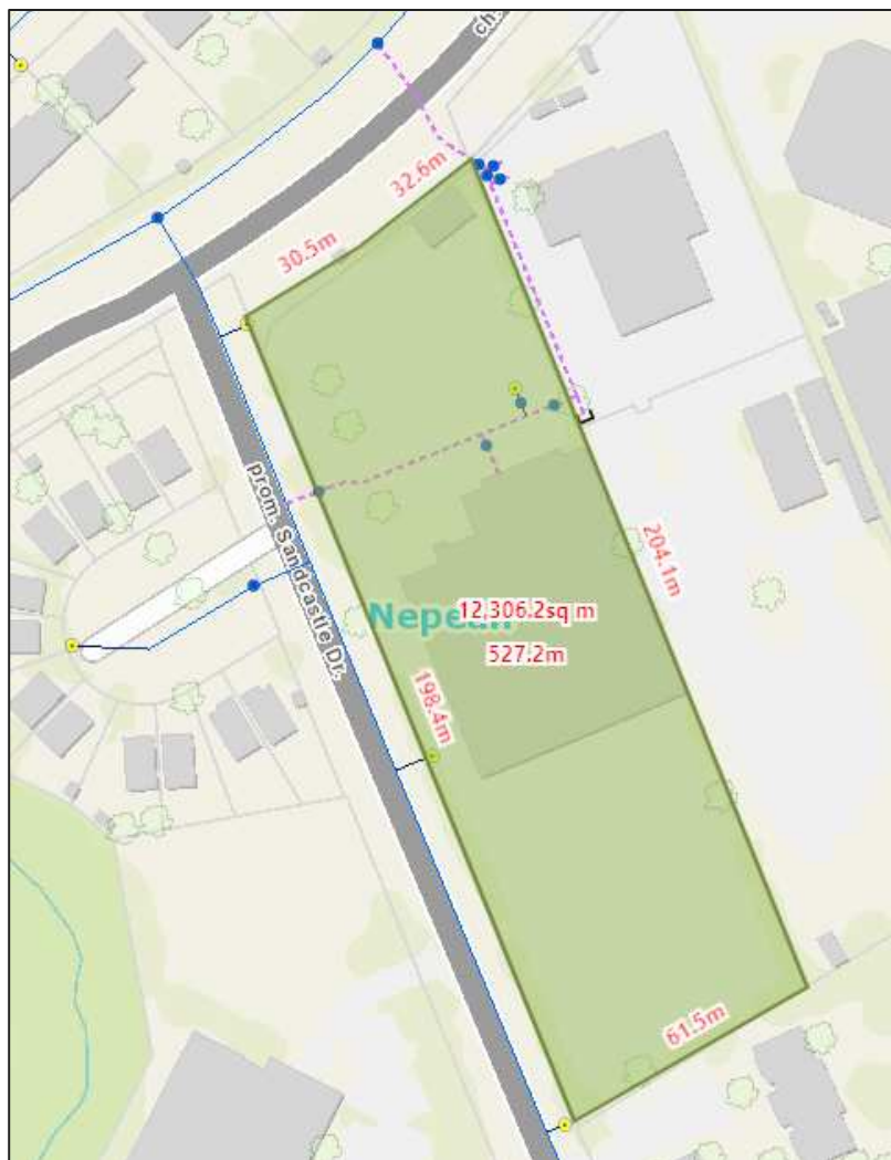
Figure 3-1: Fire Hydrant Coverage Sketch
