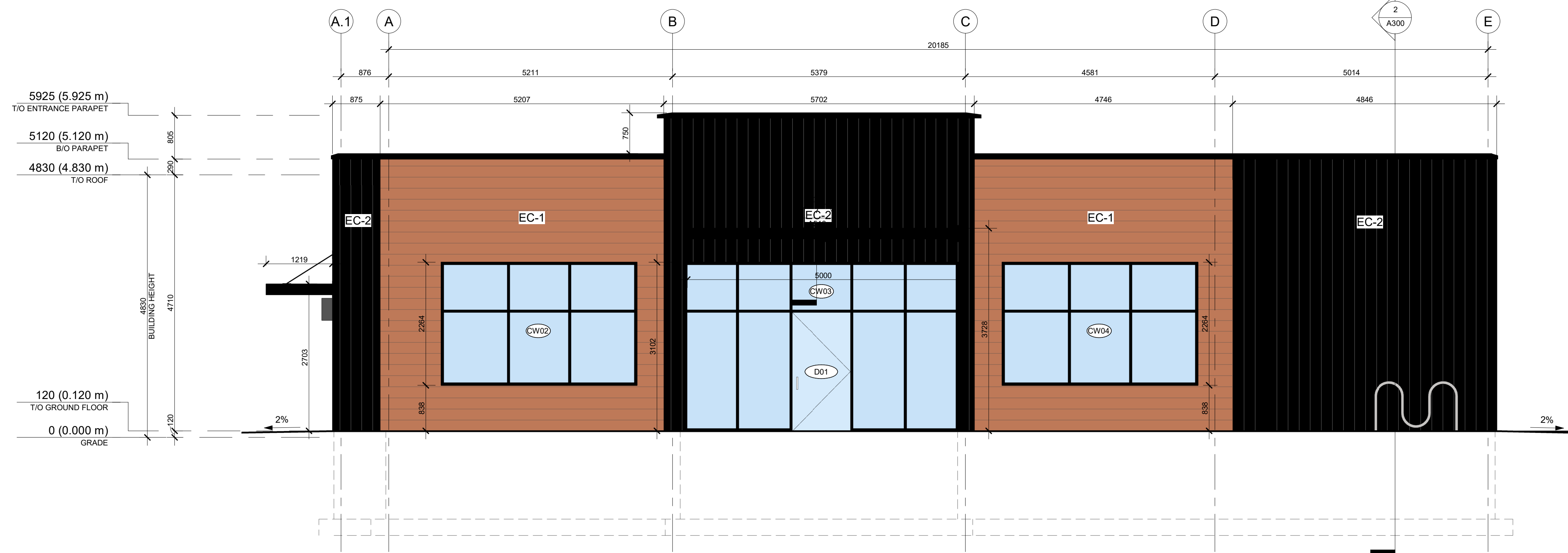
1 NORTH ELEVATION - DRIVE THRU A200 1: 50
