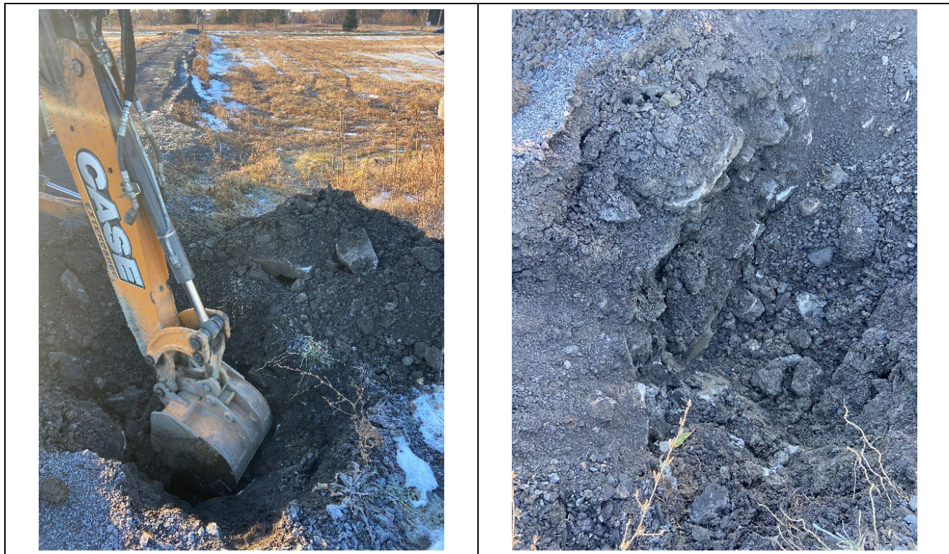
Sample SS-1 submitted for Reg 153 metals, PHC F1-F4, CN, EC, SAR and pH analysis. Samples SS-3 submitted for corrosivity analysis.
