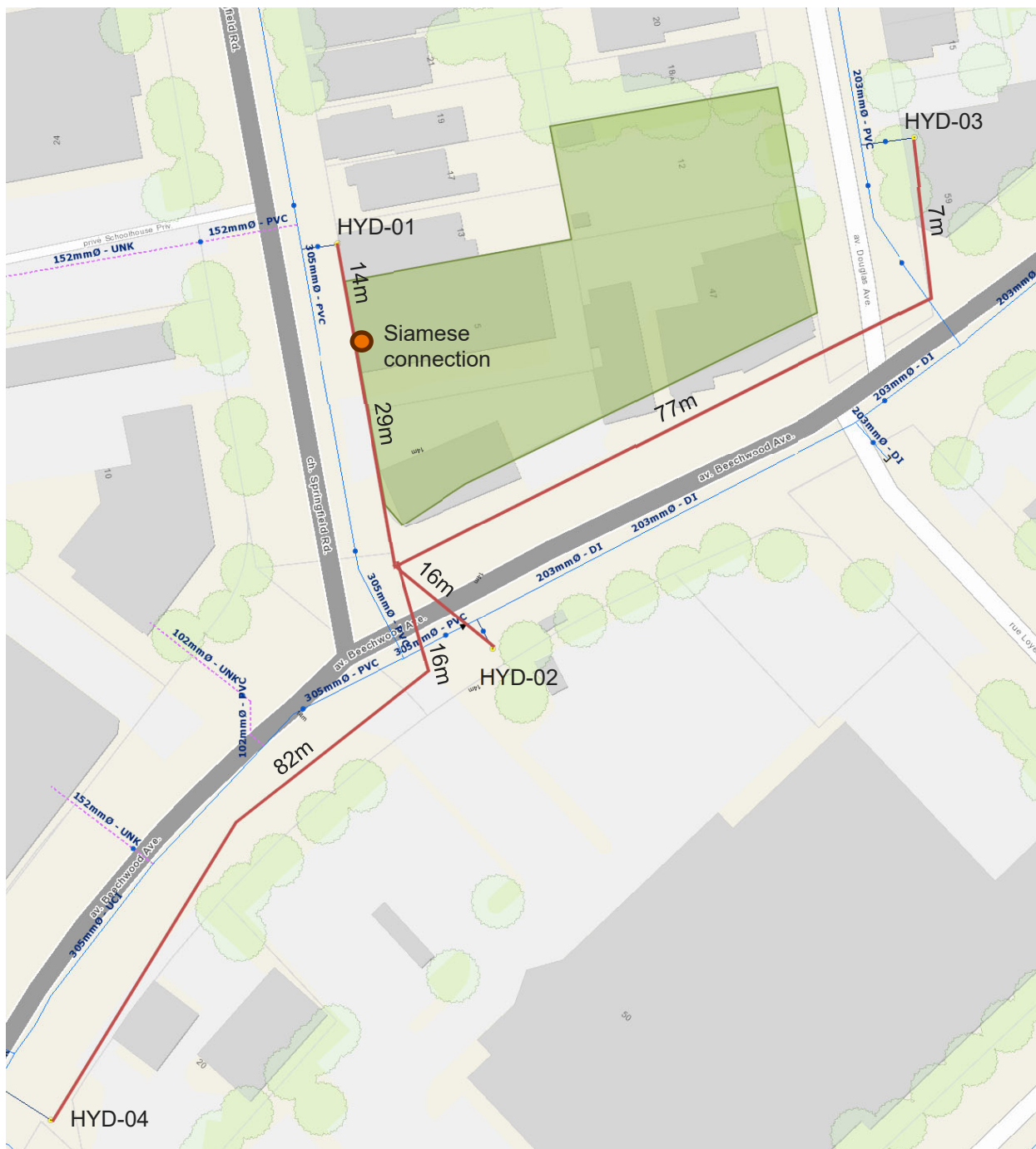
Figure 3-1: Fire Hydrant Coverage Sketch
