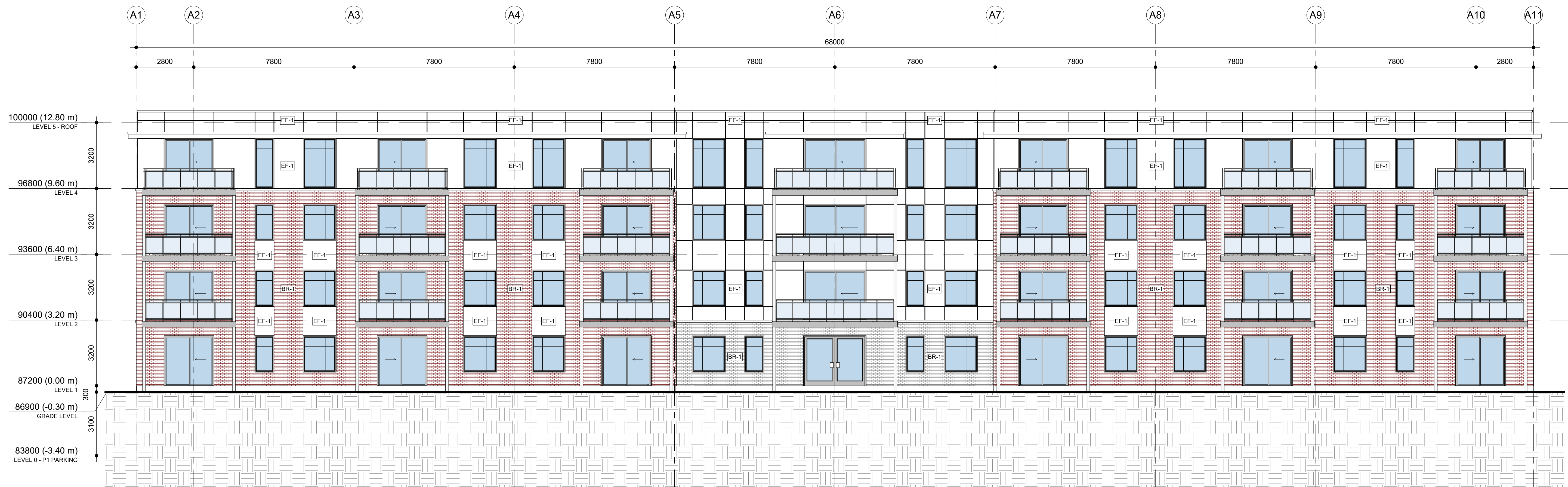
1 BUILDING A - WEST ELEVATION A200 1 : 100
