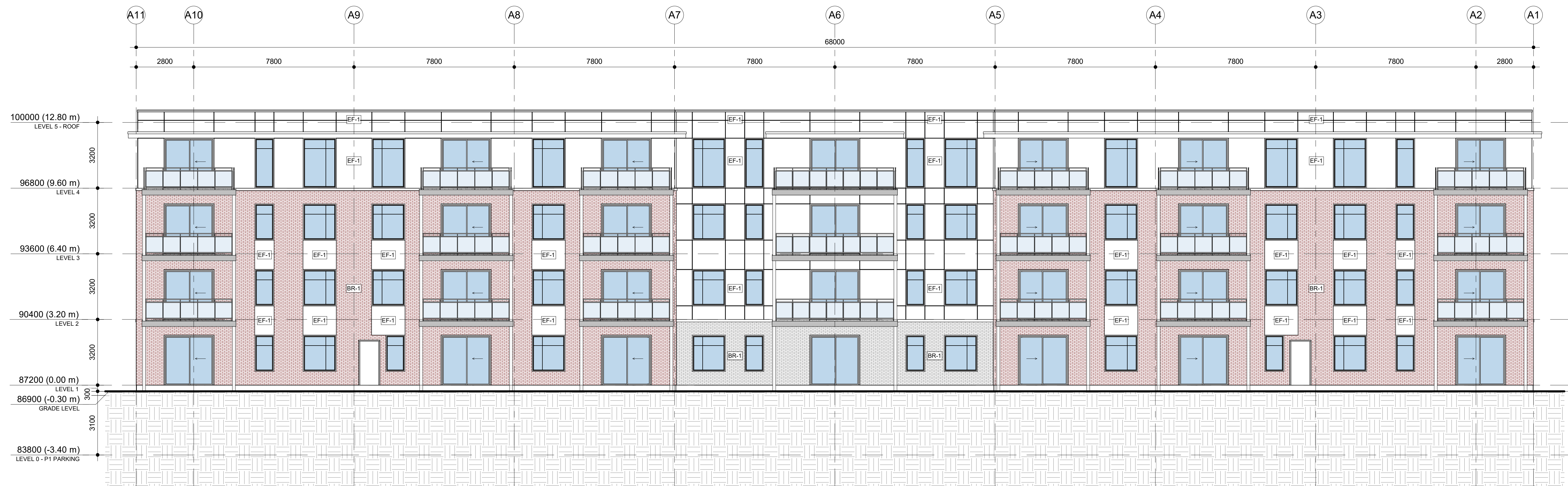
2 BUILDING A - EAST ELEVATION A200 1 : 100
